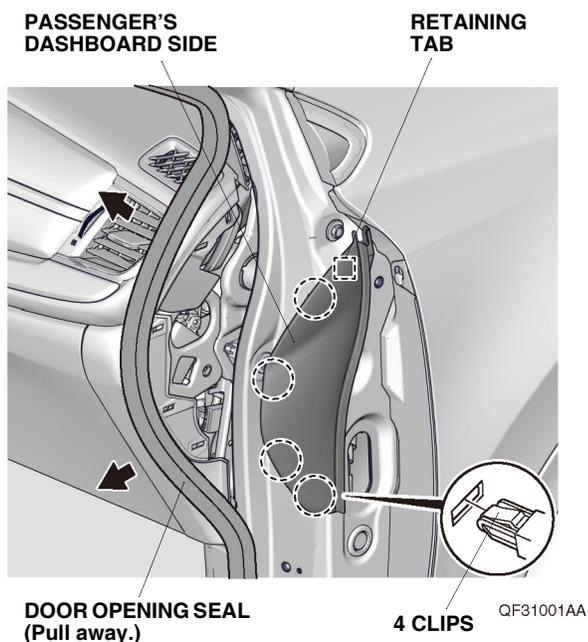
3. Remove the passenger's dashboard under cover.
