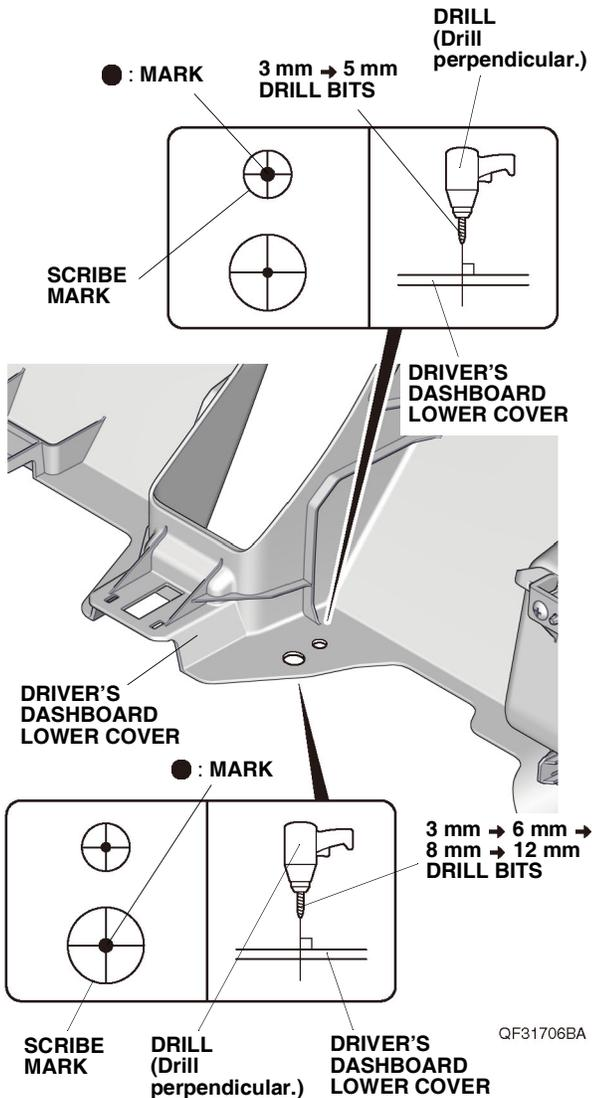
32. While wearing eye protection, drill the pierced mark on the driver's dashboard lower cover to 12 mm. First drill with a 3 mm drill bit, next drill with a 6 mm drill bit and an 8 mm drill bit, and finish with a 12 mm drill bit. Remove any burrs.
