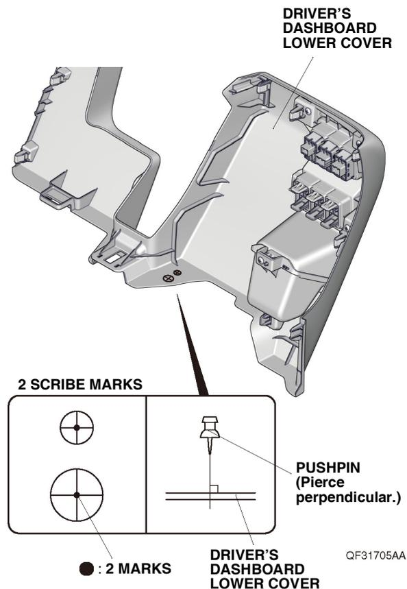
31. While wearing eye protection, drill the pierced mark on the driver's dashboard lower cover to 5 mm. First drill with a 3 mm drill bit and finish with a 5 mm drill bit. Remove any burrs.
