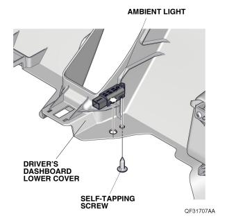
34. Plug the ambient light harness 4-pin connector into the ambient light, then install the driver's dashboard lower cover.
