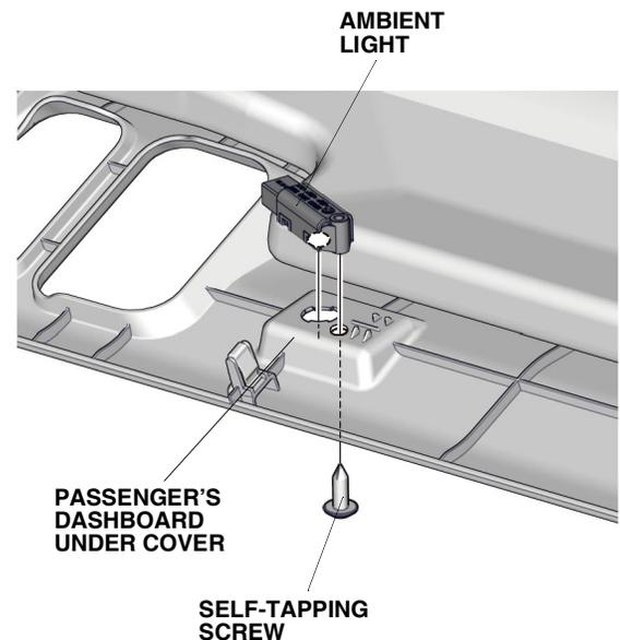
38. Install the glove box. Plug the ambient light harness 4-pin connector into the ambient light, then install the passenger's dashboard under cover.
