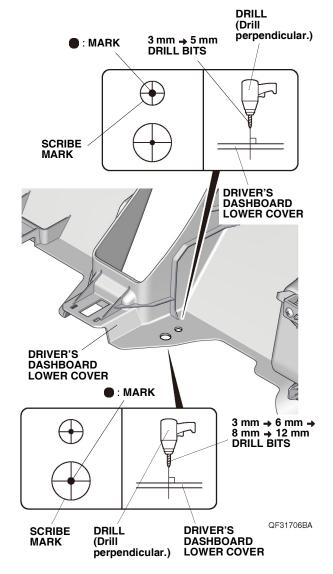
32. While wearing eye protection, drill the pierced mark on the driver's dashboard lower cover to 12 mm. First drill with a 3 mm drill bit, next drill with a 6 mm drill bit and an 8 mm drill bit, and finish with a 12 mm drill bit. Remove any burrs.
