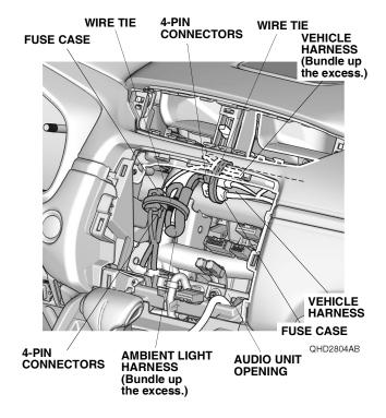
17. Bundle up the excess ambient light harness. Secure the 4-pin connectors, fuse case, and ambient light harness to the vehicle harness with one wire tie as shown. Go to step 22.
