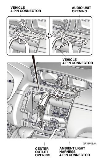
20. Plug the vehicle 4-pin connector into the ambient light harness 4-pin connector.
