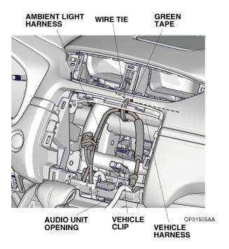
19. Route the vehicle 4-pin connector and ambient light harness 4-pin connector as shown.
