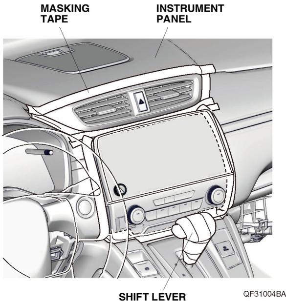
9. Remove the center outlet, and unplug the vehicle connector.
