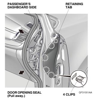
3. Remove the passenger's dashboard under cover.
