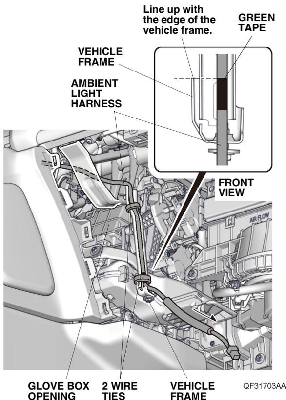
29. Secure the ambient light harness to the vehicle harness and vehicle frame with two wire ties.
