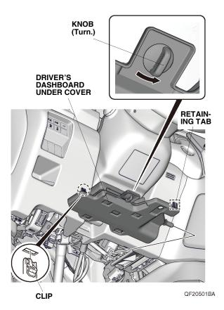
7. Pull away the door opening seal. Remove the driver's dashboard lower cover, and unplug the vehicle connectors.
