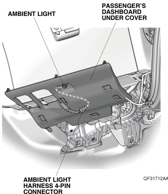
39. Install the audio unit and climate control unit. Plug the ambient light harness 4-pin connector or instrument panel illumination harness 4-pin connector into the center outlet, then install the center outlet.
