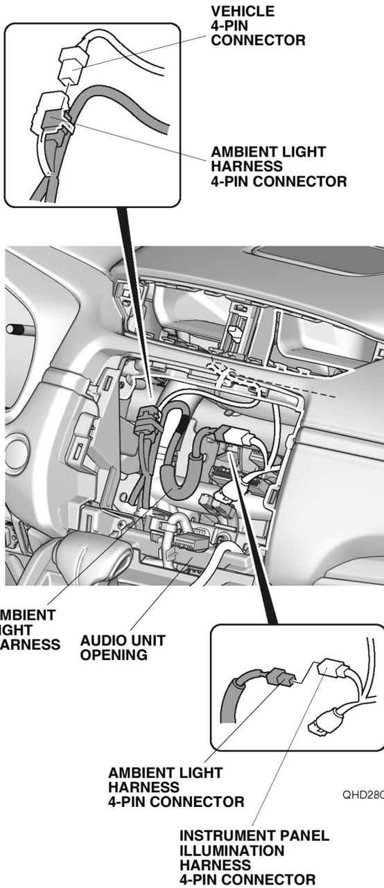
15. Plug the ambient light harness 4-pin connector into the instrument panel illumination harness 4-pin connector.
