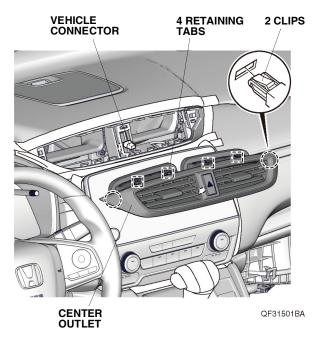
Remove the climate control unit, and unplug the vehicle connector.
