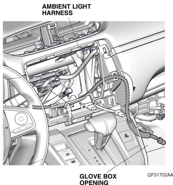
28. Line up the green tape on the ambient light harness with the edge of the vehicle frame as shown. Secure the ambient light harness to the vehicle frame with two wire ties.
