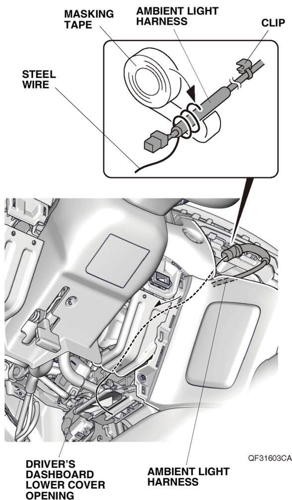
24. Lower and pull out the steering wheel. Route the ambient light harness as shown. Remove the masking tape and steel wire. Secure the ambient light harness to the vehicle panel with one clip on the ambient light harness.
