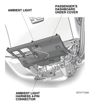
39. Install the audio unit and climate control unit. Plug the ambient light harness 4-pin connector or instrument panel illumination harness 4-pin connector into the center outlet, then install the center outlet.
