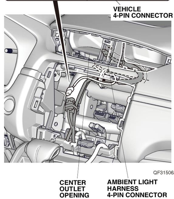
20. Plug the vehicle 4-pin connector into the ambient light harness 4-pin connector.
