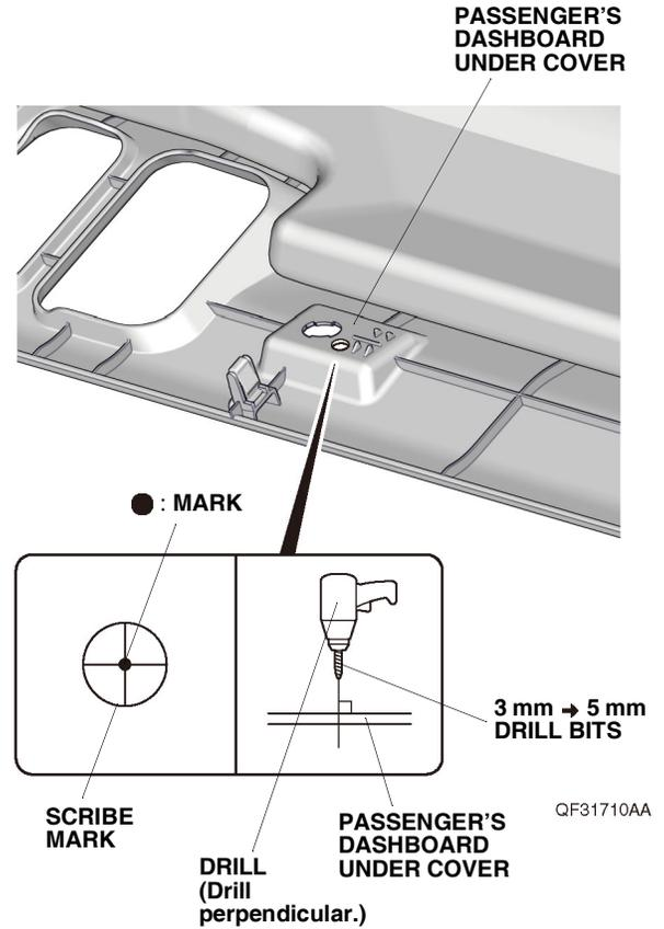
37. Install the ambient light to the passenger's dashboard under cover with one self-tapping screw.
