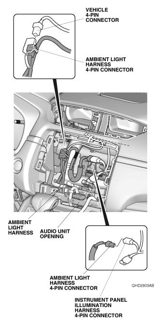
15. Plug the ambient light harness 4-pin connector into the instrument panel illumination harness 4-pin connector.
