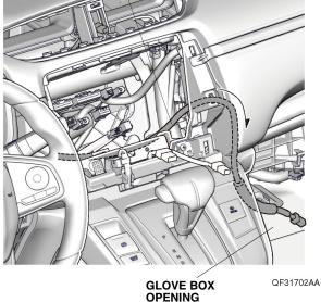
28. Line up the green tape on the ambient light harness with the edge of the vehicle frame as shown. Secure the ambient light harness to the vehicle frame with two wire ties.
