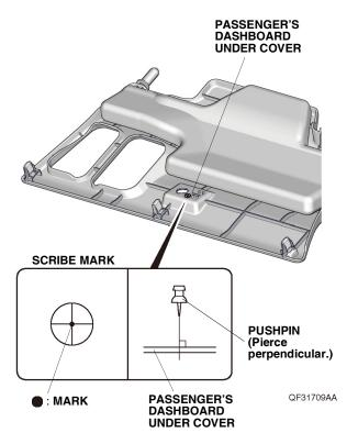
36. While wearing eye protection, drill the pierced mark on the passenger's dashboard under cover to 5 mm. First drill with a 3 mm drill bit and finish with a 5 mm drill bit. Remove any burrs.
