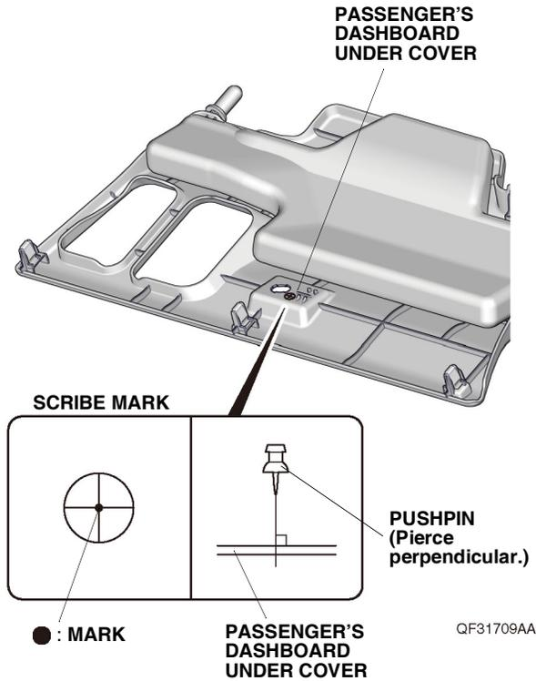
36. While wearing eye protection, drill the pierced mark on the passenger's dashboard under cover to 5 mm. First drill with a 3 mm drill bit and finish with a 5 mm drill bit. Remove any burrs.
