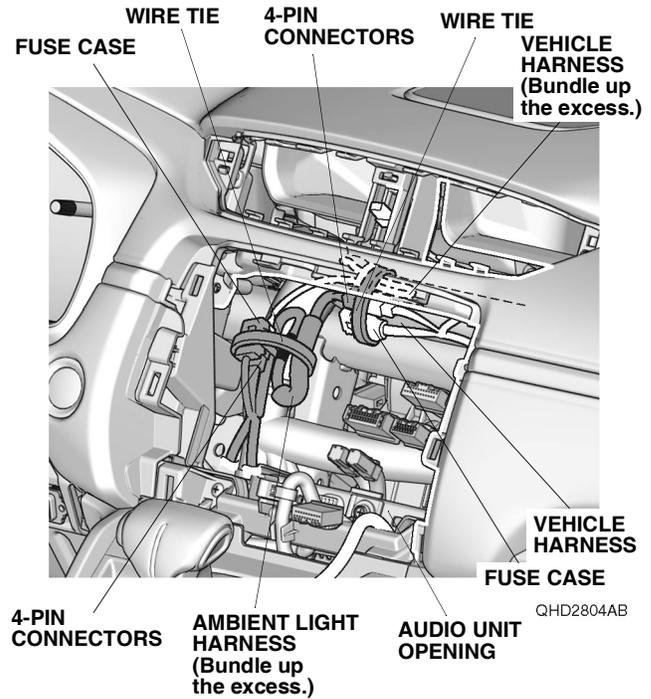
17. Bundle up the excess ambient light harness. Secure the 4-pin connectors, fuse case, and ambient light harness to the vehicle harness with one wire tie as shown. Go to step 22.
