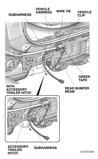
44. With the help of an assistant, bring the rear bumper close to the vehicle, and plug the subharness 3-pin connector into the hands-free access unit. Install the rear bumper.
