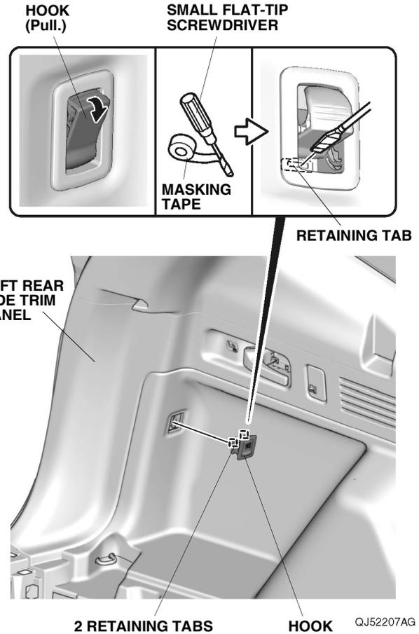
24. Apply masking tape to the left rear side trim panel as shown.
