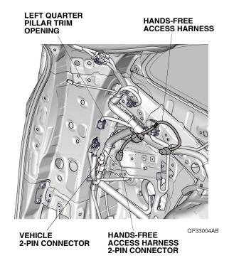
49. Line up the green tape on the hands-free access harness to the vehicle clip, and secure the hands-free access harness to the vehicle harness with one wire tie.
