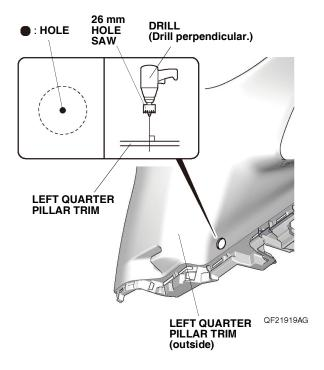
55. Install the switch into the 26 mm hole in the left guarter pillar trim.
