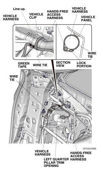
50. Secure the hands-free access harness to the vehicle harness with one wire tie.
