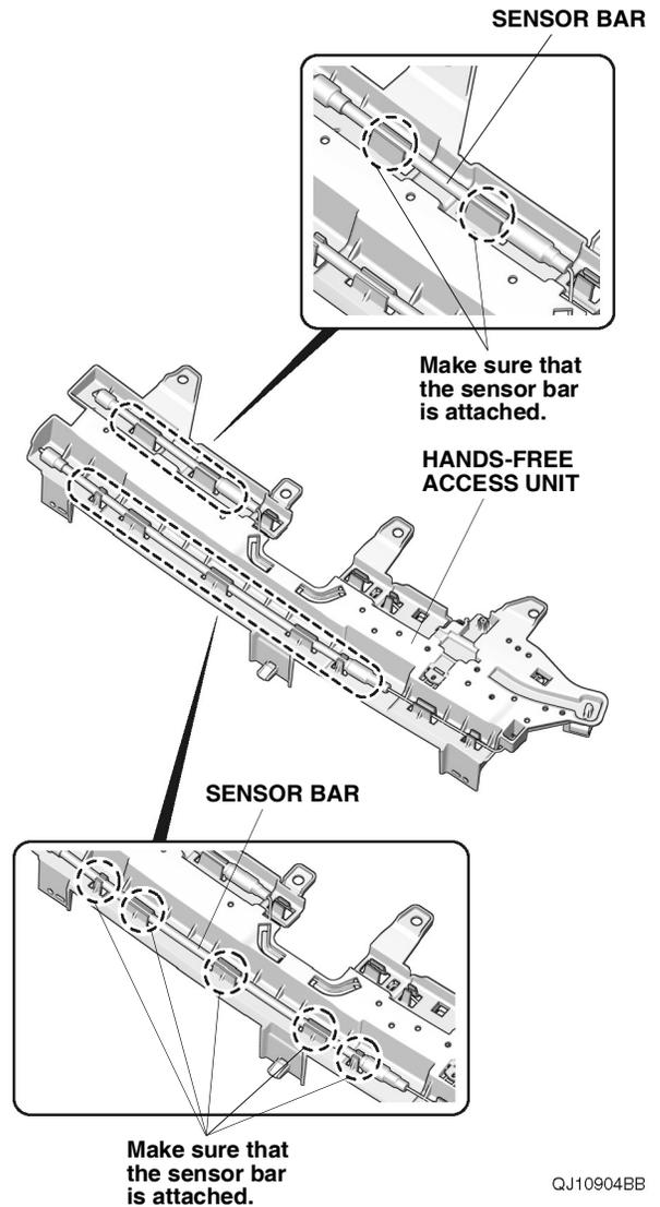
40. Install the hands-free access unit to the rear bumper with two self-tapping screws, three bumper clips A, one bumper clip B and one clip.
