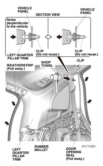
29. Using a rubber mallet wrapped with a shop towel, lightly tap the area marked **SIDE CURTAIN AIRBAG** on the left quarter pillar trim to push in the clip. Make sure to strike the area perpendicular to the vehicle.
