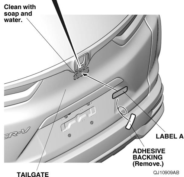
68. Remove the adhesive backing from the label A. Using the arrows on the label A, center it 5 mm (0.20 in.) below the tailgate trim and attach it to the tailgate.
