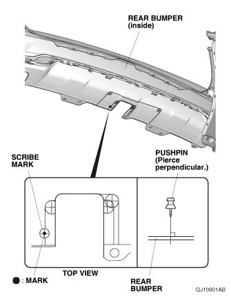
37. While wearing eye protection, drill the pierced mark on the rear bumper with a 3 mm drill bit. NOTE: Make sure to drill perpendicular to the rear bumper.
