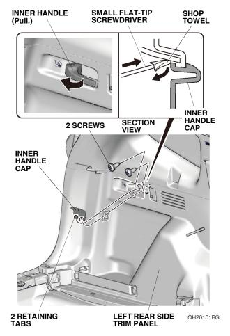
Remove the two screws from the left rear side trim panel. 12. Gently pull the hook on the left rear side trim panel, and use a small flat-tip screwdriver wrapped with masking tape to remove the hook as shown. Then, remove the two clips from the left rear side trim panel.
