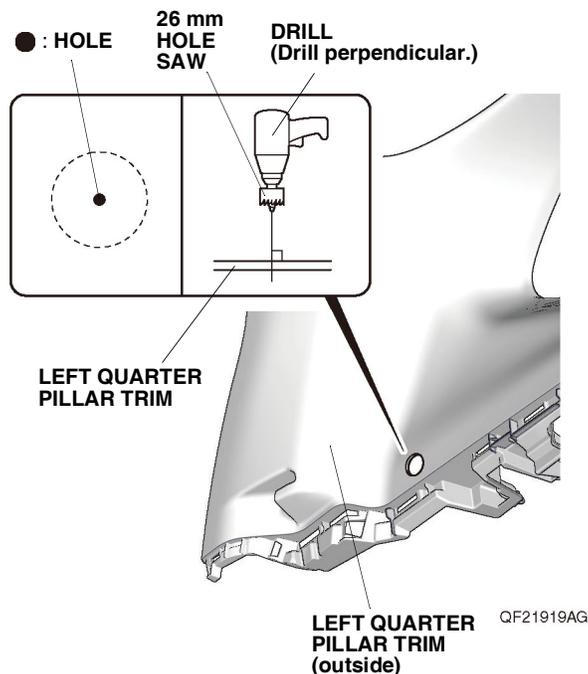
55. Install the switch into the 26 mm hole in the left quarter pillar trim.
