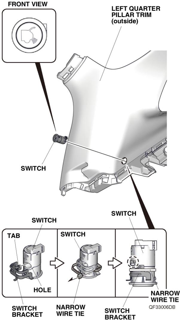
56. Line up the tab on the switch bracket with the hole on the switch, and secure the switch bracket to the switch with one narrow wire tie.
