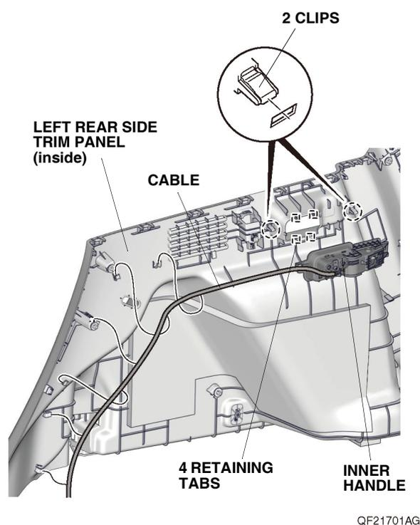
14. Pull away the door opening seal and weatherstrip from around the left rear side trim panel. Remove the left rear side trim panel, and unplug the vehicle connector.
