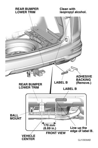
46. Remove the adhesive backing from the label B, and attach the label B to the rear bumper lower trim at the measurement shown.
