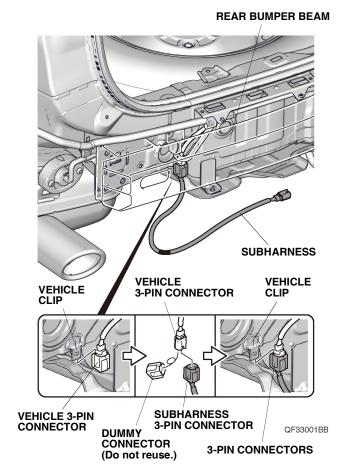
42. Plug the vehicle 3-pin connector into the subharness 3-pin connector, and secure the 3-pin connectors to the vehicle clip.
