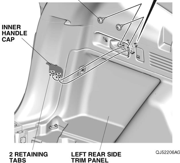
22. Remove the two screws from the left rear side trim panel.
