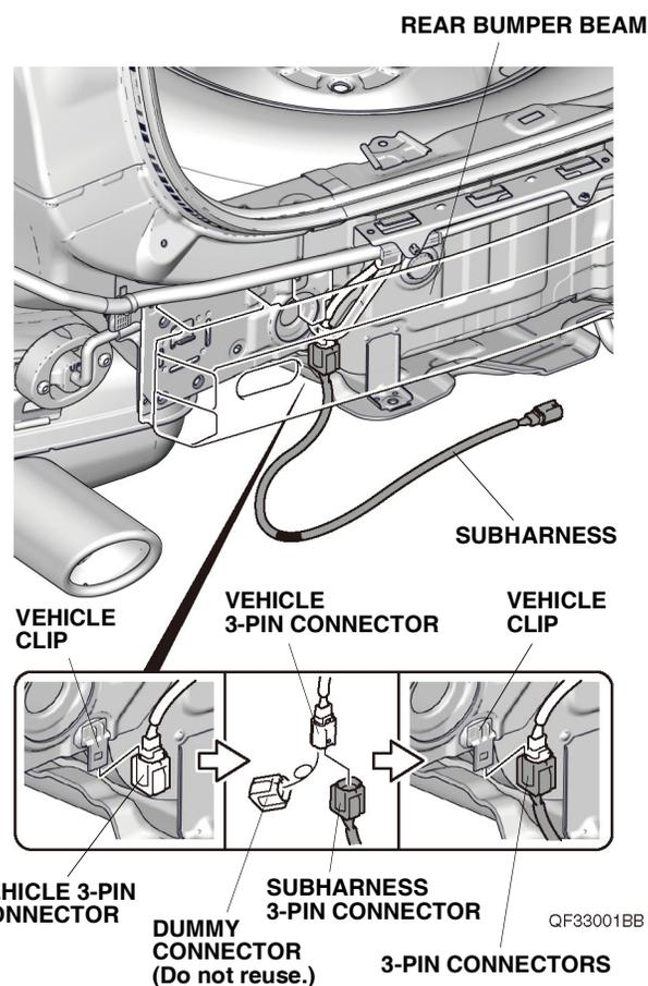
42. Plug the vehicle 3-pin connector into the subharness 3-pin connector, and secure the 3-pin connectors to the vehicle clip.
