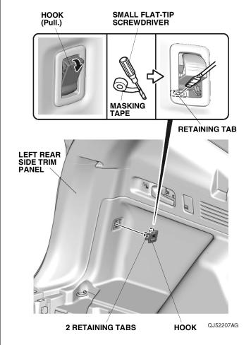
24. Apply masking tape to the left rear side trim panel as shown.
