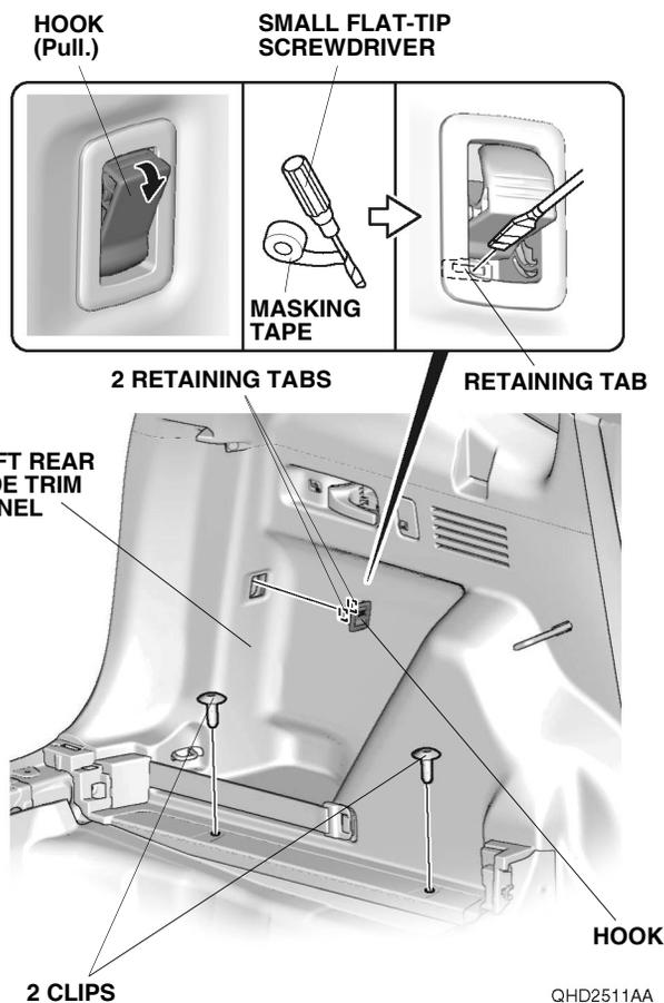
13. Apply masking tape to the left rear side trim panel as shown.
