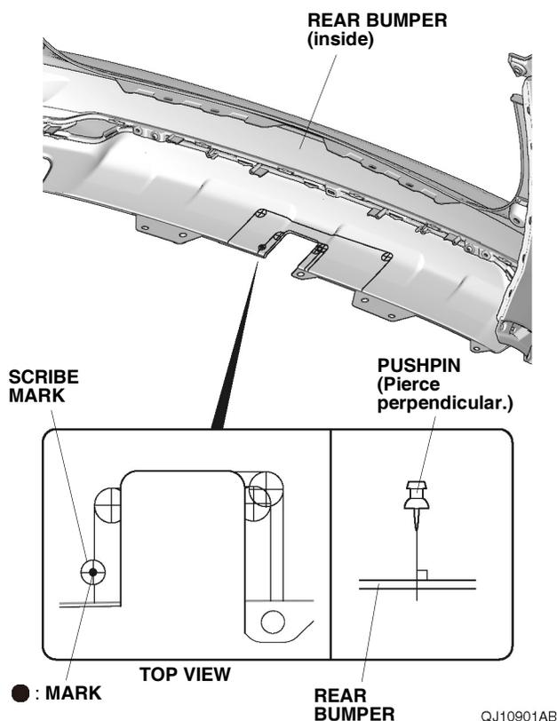
37. While wearing eye protection, drill the pierced mark on the rear bumper with a 3 mm drill bit.
