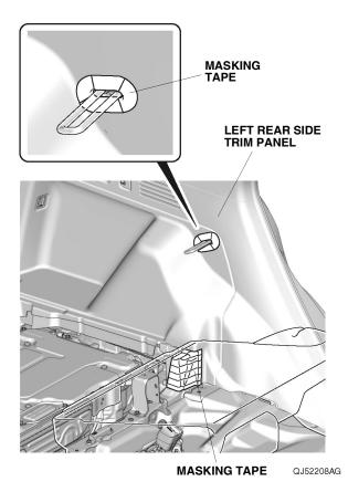
25. Pull away the door opening seal and weatherstrip from around the left rear side trim panel. Remove the left rear side trim panel, and unplug the vehicle connector.
