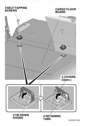
17. Remove the cargo floor board.
