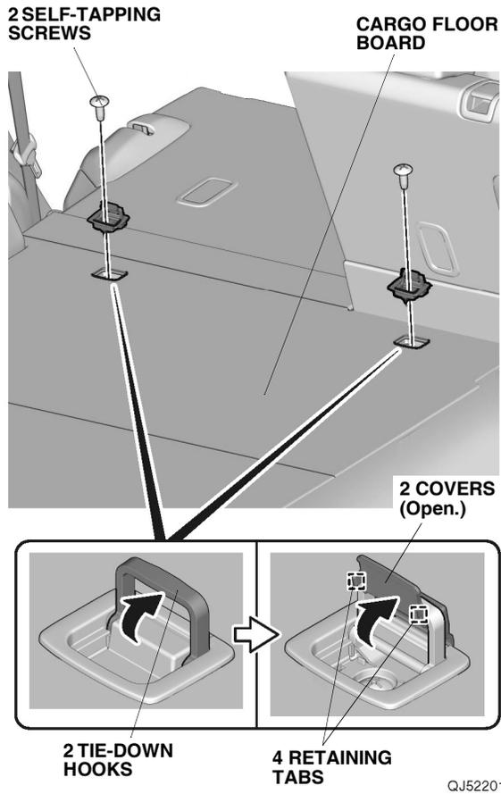
17. Remove the cargo floor board.
