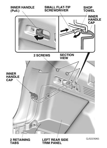
22. Remove the two screws from the left rear side trim panel.
