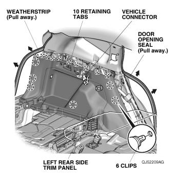
26. Release the cable from the left rear side trim panel, then remove the inner handle.
