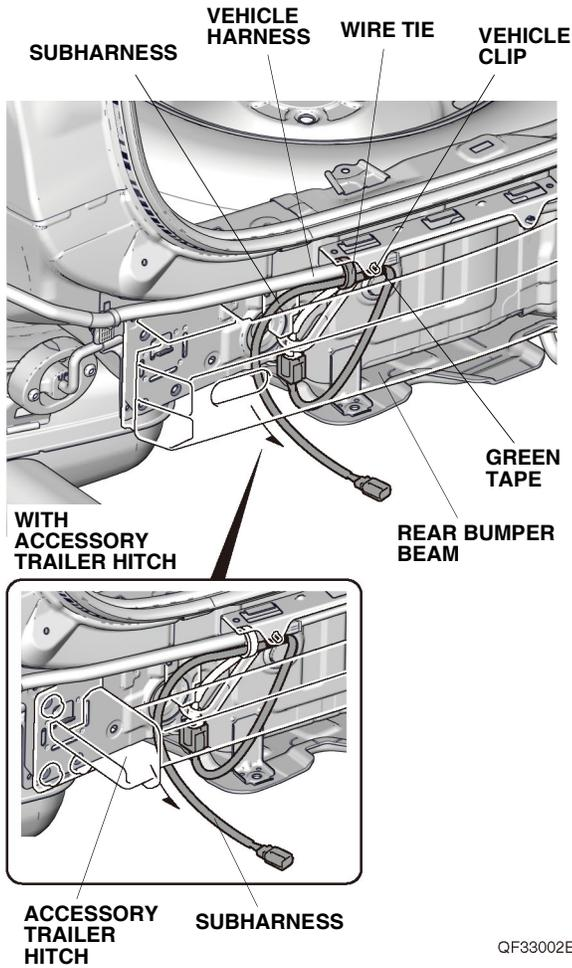
44. With the help of an assistant, bring the rear bumper close to the vehicle, and plug the subharness 3-pin connector into the hands-free access unit. Install the rear bumper.
