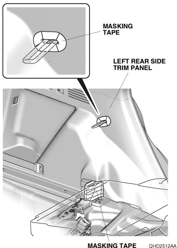
15. Release the cable from the left rear side trim panel, then remove the inner handle. Go to step 27.
