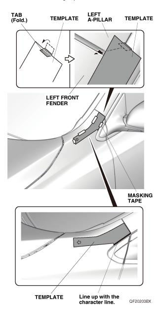
Peel back the adhesive backings, and tape them to the front surface of the left front fender trim with masking tape. Remove the remaining adhesive backings.
