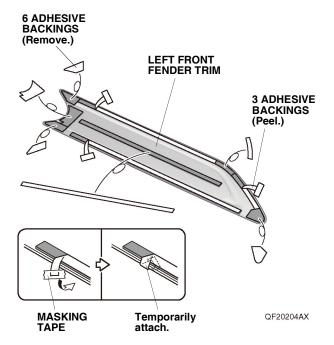
4. Line up the left front fender trim with the template, and attach it to the left front fender as shown.
