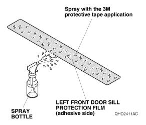
6. Line up the left front door sill protection film with the curve end and masking tape as shown. Attach the left front door sill protection film to the vehicle panel.
