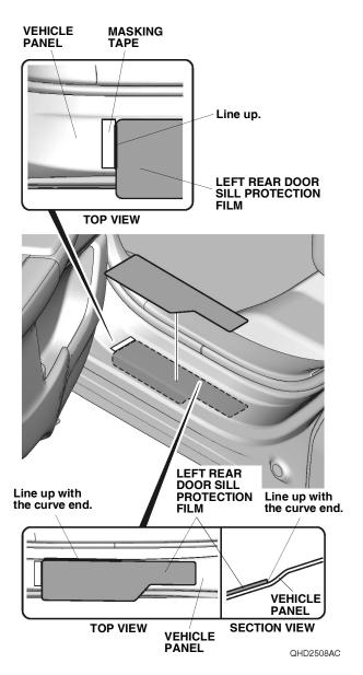
19. Starting from the inside and working outside, use the felt sleeve to smooth out the center of the left rear door sill protection film. Move the felt sleeve in one direction only. If you see an air bubble, stop and gently peel up that section to work out the bubble. Work slowly, and keep pressure against the left rear door sill protection film.
