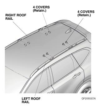
2. Position the front crossbar onto the left and right roof rails, and adjust the right stay in or out until it fits securely into position.
