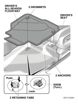
2. Place the grommets in the driver's all-season floor mat over the anchors. Push the grommets into the anchors to secure the retaining tabs, then turn the knobs 90° to secure the driver's all-season floor mat.
