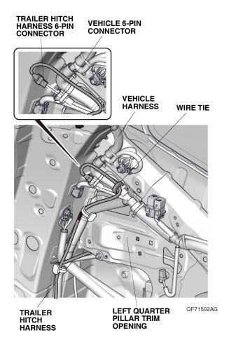
69. Secure the trailer hitch harness to the vehicle harness with one wire tie.
