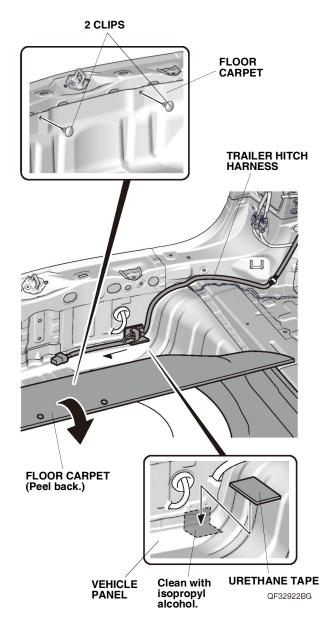
74. Using isopropyl alcohol on a shop towel, thoroughly clean the vehicle panel where the urethane tape will attach. Attach the urethane tape to the vehicle panel as shown.
