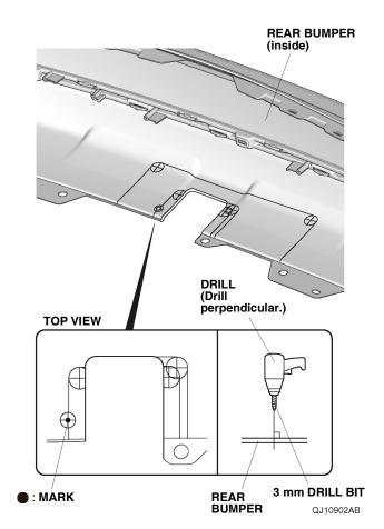
38. While wearing eye protection, enlarge the 3 mm hole to 14 mm using a 14 mm hole saw. Remove any burrs.
