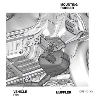
27. Remove the mounting rubber from the left side of the vehicle the same way, if equipped.
