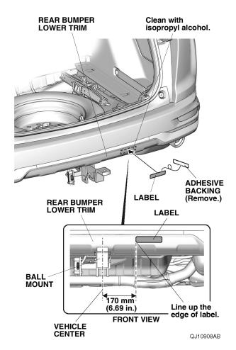
83. Remove the adhesive backing from the label, and attach the label to the rear bumper lower trim as shown.
