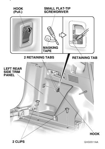
13. Apply masking tape to the left rear side trim panel as shown.
