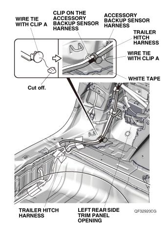
71. Line up the white tape on the trailer hitch harness with the clip on the accessory backup sensor harness, and secure the trailer hitch harness to the accessory backup sensor harness with one wire tie with clip A. Go to step 73.
