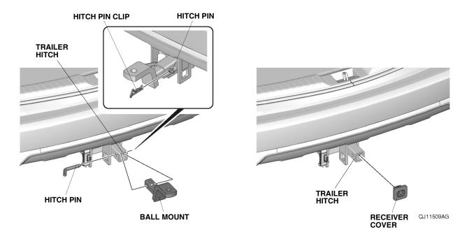
After the first 600 miles (1,000 km) of towing, have your Honda dealer check the tightness of the trailer hitch bolts.
