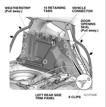
15. Release the cable from the left rear side trim panel, then remove the inner handle.
