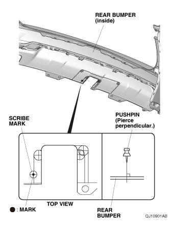
While wearing eye protection, drill the pierced mark on the rear bumper with a 3 mm drill bit. NOTE: Make sure to drill perpendicular to the rear bumper.
