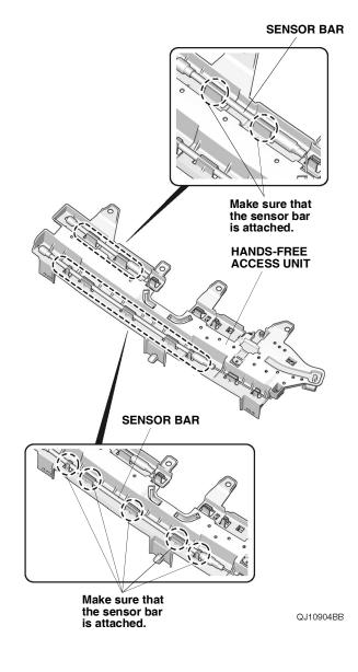
40. Install the hands-free access unit to the rear bumper with two self-tapping screws, three clips A removed in step 31, one bumper clip B, and one clip.
