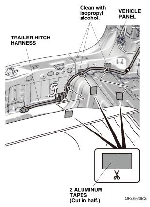
76. Using scissors, cut the two pieces of aluminum tape in half, and secure the trailer hitch harness to the vehicle panel with three halves of aluminum tape as shown. 77. Plug the trailer hitch harness 4-pin connector into the socket harness 4-pin connector.
