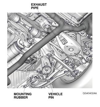
30. Using a utility knife, cut off the rear under cover as shown. Remove any burrs and sharp edges from the corners.
