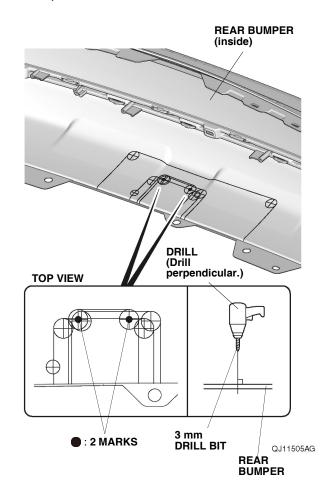
34. While wearing eye protection, enlarge the 3 mm holes to 20 mm using a 20 mm hole saw.NOTE: Make sure to drill perpendicular to the rear bumper.
