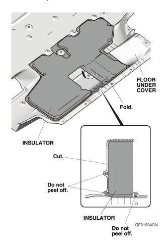
4. Using a utility knife, cut off the floor under cover as shown.
