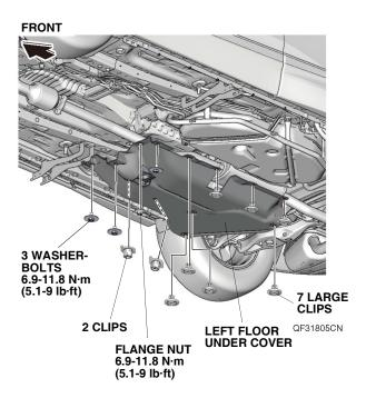
23. Install the right floor under cover. Torque the flange nut and washer-bolts to 6.9-11.8 N·m (5.1-9 lb·ft).
