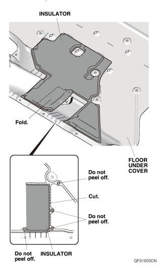
3. Using a utility knife, cut the insulator on the floor under cover and fold it into the inside of the insulator as shown.
