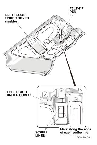
12. Using a utility knife, cut the left floor under cover as shown.
