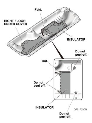
Using a utility knife, cut off the right floor under cover as shown.
