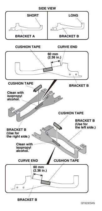
17. Attach one cushion tape to each bracket B as shown. Make sure to attach the cushion tapes in the correct position and orientation.
