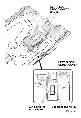
13. Using a felt-tip pen, mark the left floor under cover as shown.
