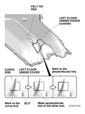
14. Using a utility knife, cut off the left floor under cover along the mark.
