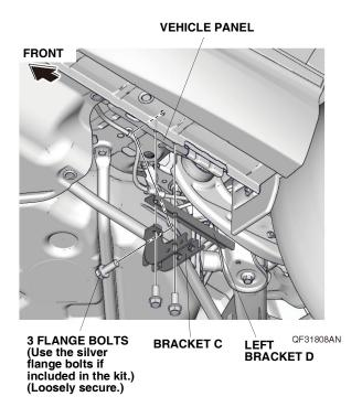
26. With the help of an assistant, loosely secure the left running board to bracket A, bracket B, bracket C, and left bracket D with 13 flange bolts.
