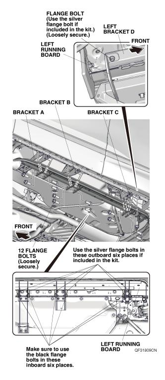
27. Secure bracket A, bracket B, and bracket C to the vehicle panel with nine flange bolts. Torque the flange bolts to 22 N·m (16 lb·ft).
