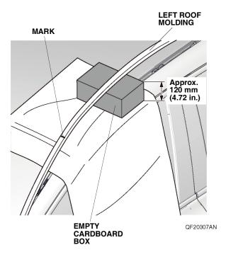
7. While wearing eye protection, use an air saw to cut the left roof molding at the mark. Do not use a cutting wheel or shears to cut the left roof molding; that can damage the left roof molding. With the help of an assistant, hold the rear edge while cutting. Remove any burrs.
