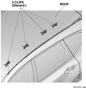
12. Using a flat-tip screwdriver wrapped with tape, remove the left roof molding cover from the left roof molding. Do not reuse the left roof molding.
