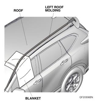
6. Place an empty cardboard box (approx. 120 mm height) under the left roof molding near the mark.
