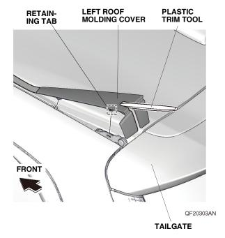
3. Pull the left roof molding toward the outside of the vehicle to release the locking tabs, and then press the locking tabs toward the inside of the vehicle, and release the left roof molding from the vehicle. When releasing the left roof molding, start from the rear of the vehicle and work toward the front.
