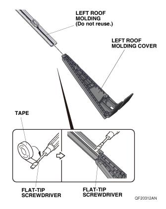
Install the left roof molding cover in its original position on the roof with one retaining tab.
