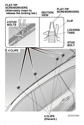
Remove four clips from the roof.
