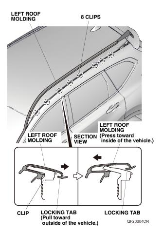
4. While pulling up the left roof molding, remove two clips. Insert a plastic trim tool alternately to each slot in the clip, and release the locking tabs in the order shown. When releasing the left roof molding, start from the rear of vehicle and work toward the front. Be careful not to deform the roof molding.
