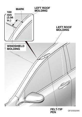
2. Using a plastic trim tool, pry up on the left roof molding cover to release one retaining tab.
