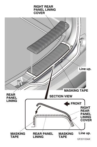
6. Using a rubber roller, apply firm pressure against the right rear panel lining cover, and roll from one end to the other. Apply firm pressure, especially at the ends.
