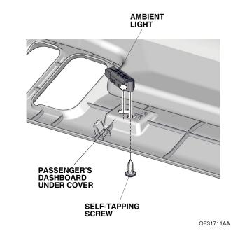
Install the glove box. Plug the ambient light harness
