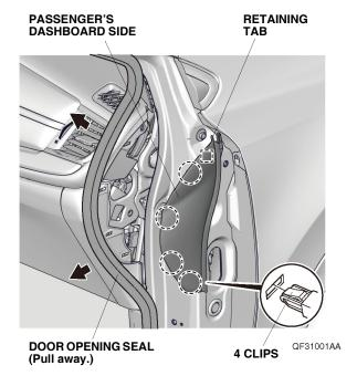
3. Remove the passenger's dashboard under cover.
