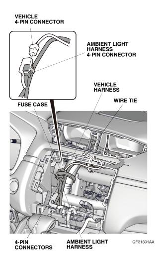
21. Secure the 4-pin connectors, fuse case, and ambient light harness to the vehicle harness with one wire tie as shown.
