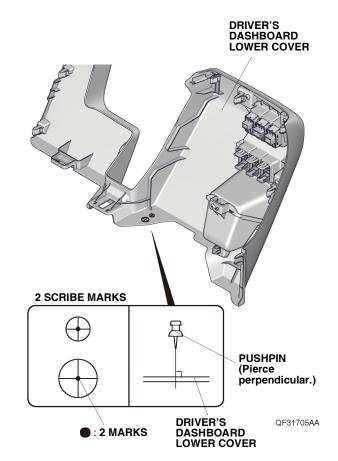
31. While wearing eye protection, drill the pierced mark on the driver's dashboard lower cover to 5 mm. First drill with a 3 mm drill bit and finish with a 5 mm drill bit. Remove any burrs.
