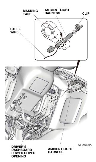
24. Lower and pull out the steering wheel. Route the ambient light harness as shown. Remove the masking tape and steel wire. Secure the ambient light harness to the vehicle panel with one clip on the ambient light harness.
