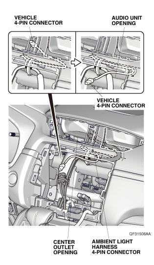
20. Plug the vehicle 4-pin connector into the ambient light harness 4-pin connector.
