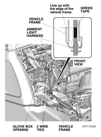
29. Secure the ambient light harness to the vehicle harness and vehicle frame with two wire ties.
