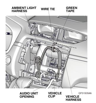
19. Route the vehicle 4-pin connector and ambient light harness 4-pin connector as shown.
