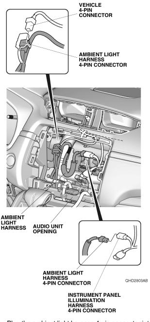
15. Plug the ambient light harness 4-pin connector into the instrument panel illumination harness 4-pin connector.
