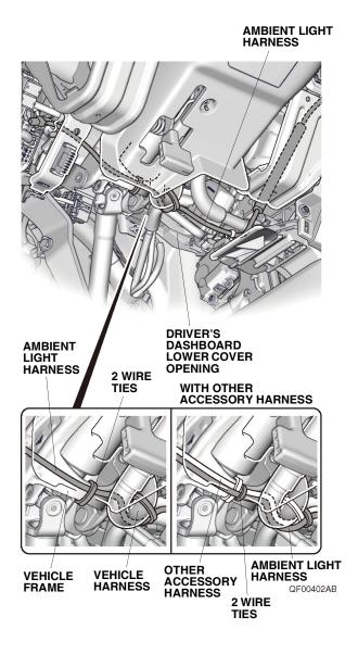
26. Secure the ambient light harness to the vehicle harness with one wire tie. Move the steering wheel up and down through its full adjustment range and make sure the ambient light harness is not being pinched or stretched.
