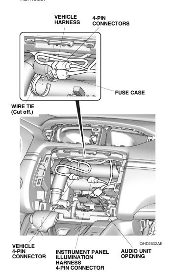
14. Plug the vehicle 4-pin connector into the ambient light harness 4-pin connector.
