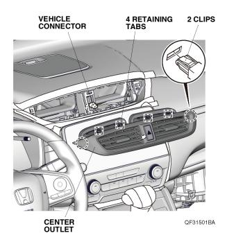
10. Remove the climate control unit, and unplug the vehicle connector.
