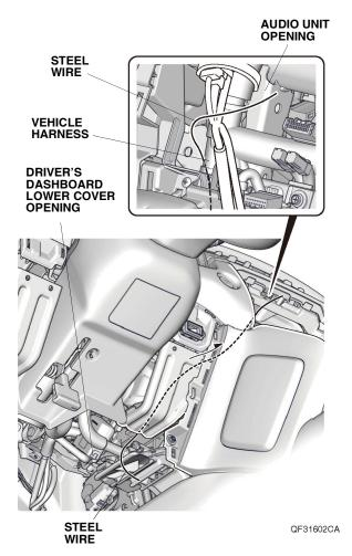
23. Attach the steel wire to the ambient light harness with masking tape and route the harness as shown.
