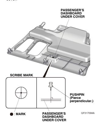
36. While wearing eye protection, drill the pierced mark on the passenger's dashboard under cover to 5 mm. First drill with a 3 mm drill bit and finish with a 5 mm drill bit. Remove any burrs. NOTE: Make sure to drill perpendicular to the passenger's dashboard under cover.
