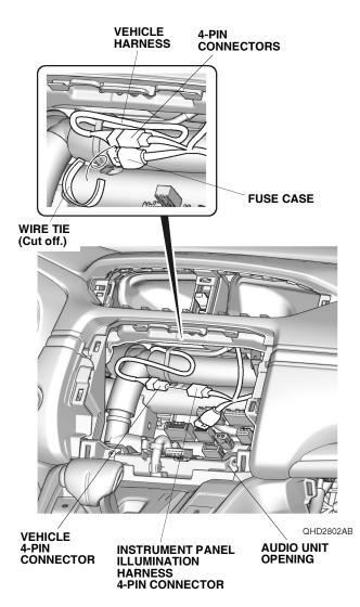
14. Plug the vehicle 4-pin connector into the ambient light harness 4-pin connector.
