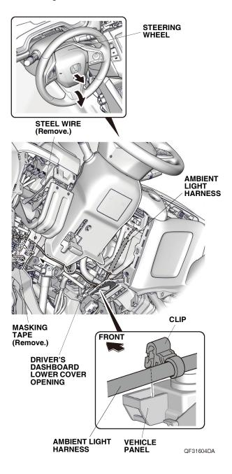
25. Secure the ambient light harness to the vehicle frame and vehicle harness with two wire ties. If the vehicle is already equipped with the other accessory harness, secure the ambient light harness to the other accessory harness with two wire ties as shown.
