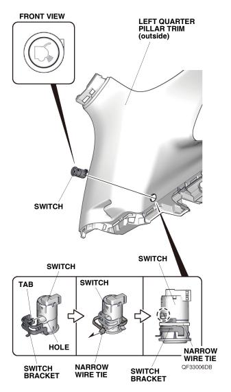
56. Line up the tab on the switch bracket with the hole on the switch, and secure the switch bracket to the switch with one narrow wire tie.
