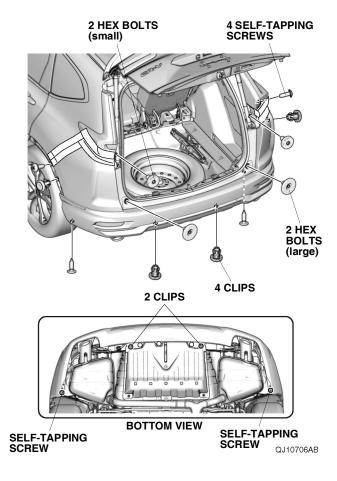
• With the help of an assistant, release the eight retaining tabs on each side.
