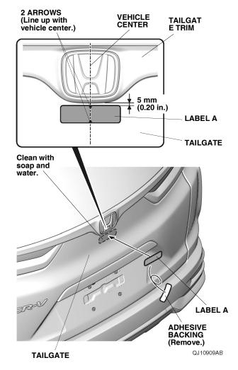
68. Remove the adhesive backing from the label A. Using the arrows on the label A, center it 5 mm (0.20 in.) below the tailgate trim and attach it to the tailgate.
