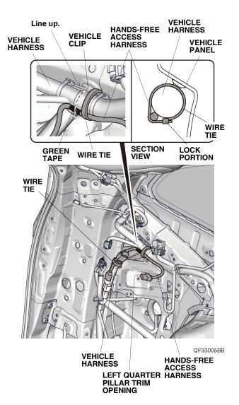
50. Secure the hands-free access harness to the vehicle harness with one wire tie.
