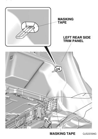
25. Pull away the door opening seal and weatherstrip from around the left rear side trim panel. Remove the left rear side trim panel, and unplug the vehicle
