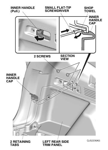
22. Remove the two screws from the left rear side trim panel.
