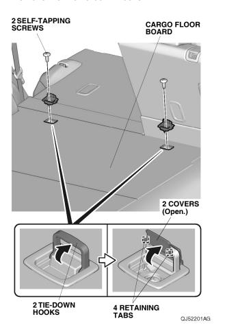
17. Remove the cargo floor board.
