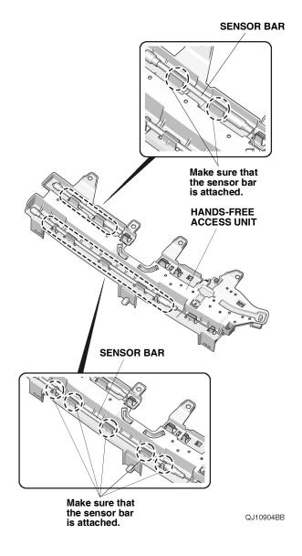
Install the hands-free access unit to the rear bumper with two self-tapping screws, three bumper clips A, one bumper clip B and one clip.
