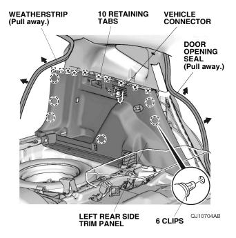
15. Release the cable from the left rear side trim panel, then remove the inner handle. Go to step 27.
