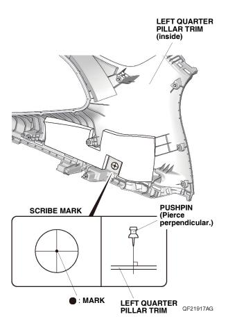
53. While wearing eye protection, drill the pierced mark on the left quarter pillar trim with a 3 mm drill bit.
