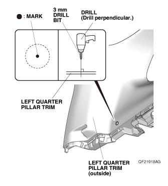
54. While wearing eye protection, enlarge the 3 mm hole to 26 mm using a 26 mm hole saw. Remove any burrs.
