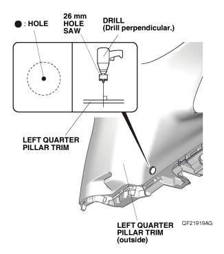
55. Install the switch into the 26 mm hole in the left quarter pillar trim.
