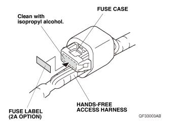
48. Plug the vehicle 2-pin connector into the hands-free access harness 2-pin connector.
