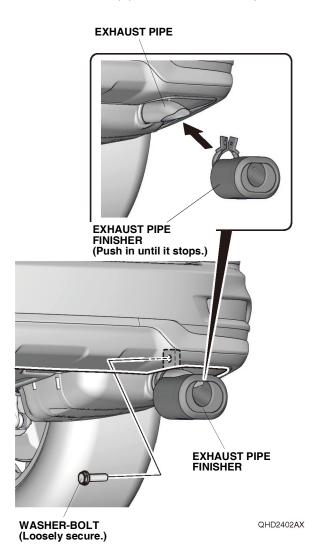
2. Loosely secure the exhaust pipe finisher to the exhaust pipe with one washer-bolt.
