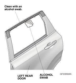
17. Peel back the adhesive backings partway and temporarily attach them to the front surface of the left rear door visor with masking tape.
