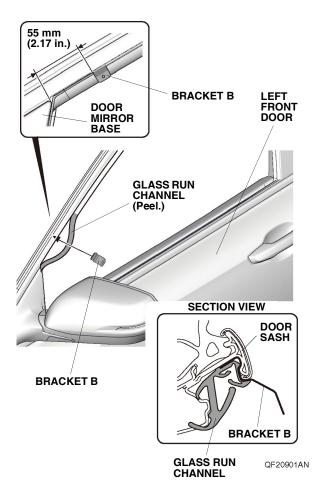
Install bracket B between the door sash and the glass run channel as shown. Seat the glass run channel properly around the bracket.
