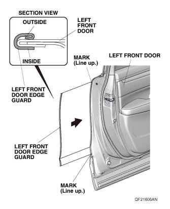
Starting at the feature line, use a rubber mallet to tap the left front door edge guard into position with a series of light taps, then work up and down. Make sure the position of the left front door edge guard is
