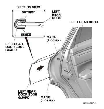
17. Starting at the feature line, use a rubber mallet to tap the left rear door edge guard into position with a series of light taps, then work up and down. Make sure the position of the left rear door edge guard is correct.
