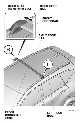
3. Secure the front crossbar to the left and right roof rails with four TORX bolts. Torque the TORX bolts to 10 N·m (lb·ft).
