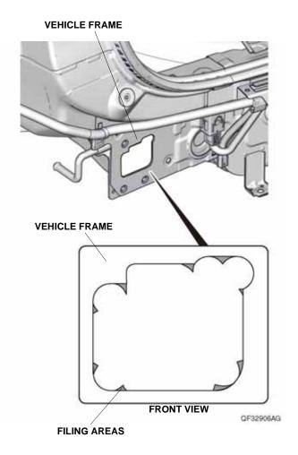
43. Apply touch-up paint to the edge of the hole. Allow the touch-up paint to dry thoroughly.
