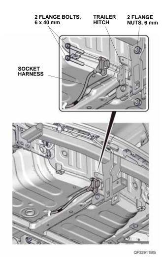
55. Line up the white tape on the socket harness with the hole on the trailer hitch, and secure the socket harness to the trailer hitch with one wire tie at the white tape on the socket harness.
