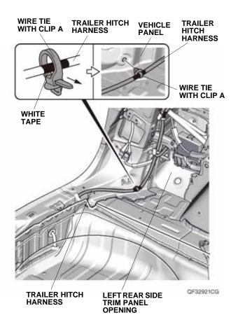
73. Peel back the floor carpet, then route the trailer hitch harness as shown.
