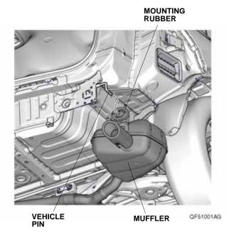
27. Remove the mounting rubber from the left side of the vehicle the same way, if equipped.
