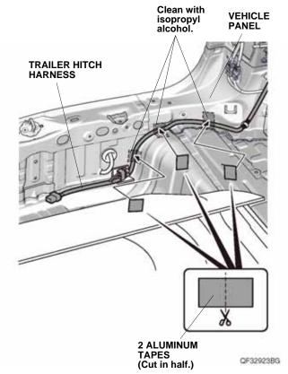
76. Using scissors, cut the two pieces of aluminum tape in half, and secure the trailer hitch harness to the vehicle panel with three halves of aluminum tape as shown.
