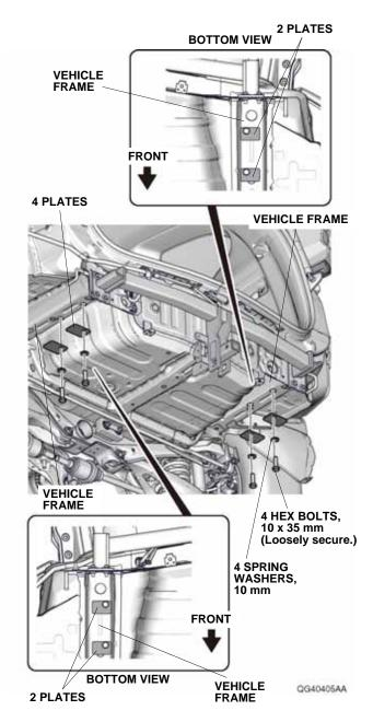
50. Loosely secure the center plate to the trailer hitch with two 12 mm plain washers, one 12 mm spring washer, one 12 mm hex nut, and one 12 x 50 mm hex bolt through the tow hook.
