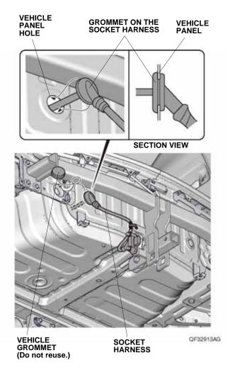
57. Install the grommet on the socket harness into the vehicle panel hole.
