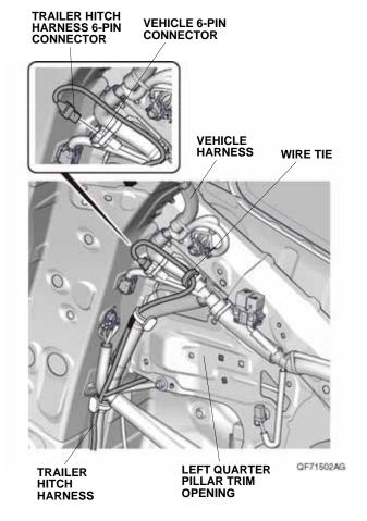
69. Secure the trailer hitch harness to the vehicle harness with one wire tie.
