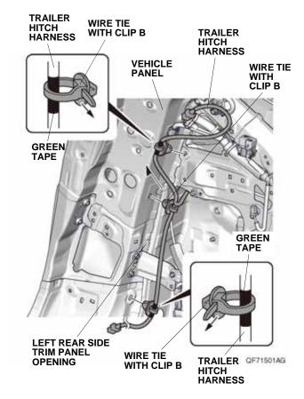
67. Secure the trailer hitch harness to the vehicle panel with one wire tie with clip B.
