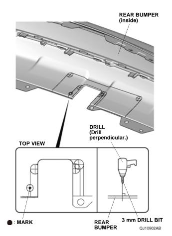
While wearing eye protection, enlarge the 3 mm hole to 14 mm using a 14 mm hole saw. Remove any burrs.
