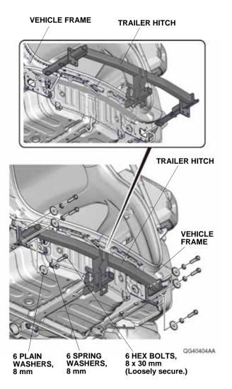
48. Loosely secure the trailer hitch to the vehicle frame with six 8 mm plain washers, six 8 mm spring washers, and six 8 x 30 mm hex bolts.
