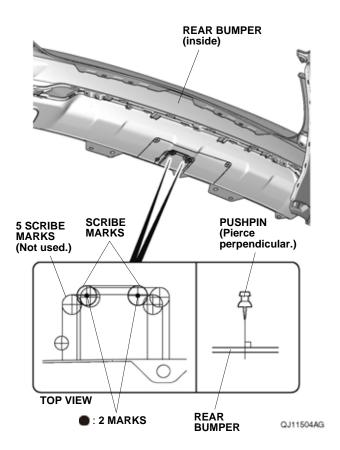
33. While wearing eye protection, drill the two pierced marks on the rear bumper with a 3 mm drill bit. NOTE: Make sure to drill perpendicular to the rear bumper.
