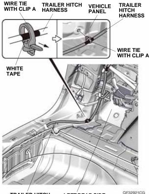
TRAILER HITCH HARNESS LEFT REAR SIDE TRIM PANEL OPENING 73. Peel back the floor carpet, then route the trailer hitch harness as shown.
