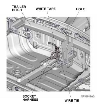
56. Remove the vehicle grommet. Route the socket harness through the vehicle panel hole.
