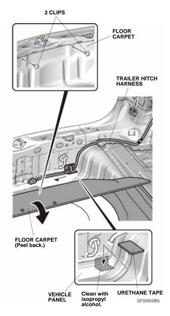
74. Using isopropyl alcohol on a shop towel, thoroughly clean the vehicle panel where the urethane tape will attach. Attach the urethane tape to the vehicle panel as shown.
