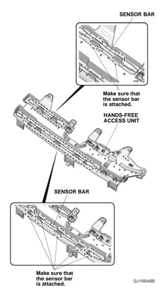
40. Install the hands-free access unit to the rear bumper with two self-tapping screws, three clips A removed in step 31, one bumper clip B, and one clip.
