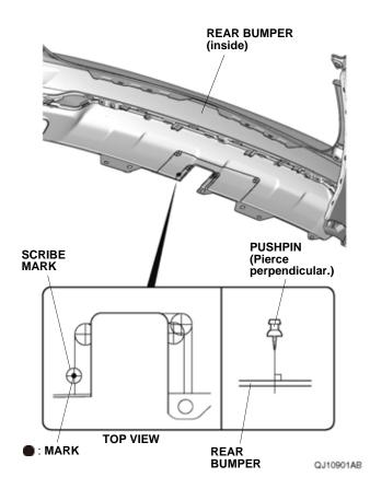
37. While wearing eye protection, drill the pierced mark on the rear bumper with a 3 mm drill bit.
