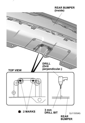
34. While wearing eye protection, enlarge the 3 mm holes to 20 mm using a 20 mm hole saw.NOTE: Make sure to drill perpendicular to the rear bumper.
