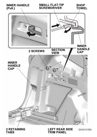
11. Remove the two screws from the left rear side trim panel.
