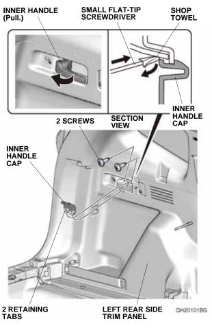
11. Remove the two screws from the left rear side trim panel.
