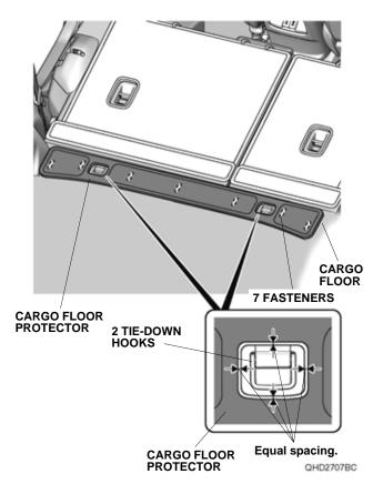
8. Check the installation condition. Make sure that the protectors do not interfere with the vehicle parts while moving the left and right rear seat-backs back and forth.
