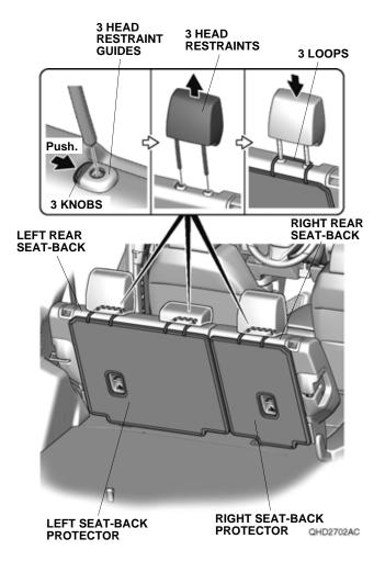
3. Fold down the left and right rear seat-backs, and peel back the left and right cargo floor lids. Line up the left and right seat-back protectors with the tether anchor covers on the left and right rear seat-backs as shown. Secure the left and right seat-back protectors to the left and right rear seat-backs with 15 fasteners.
