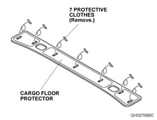
Position the cargo floor protector on the cargo floor.
