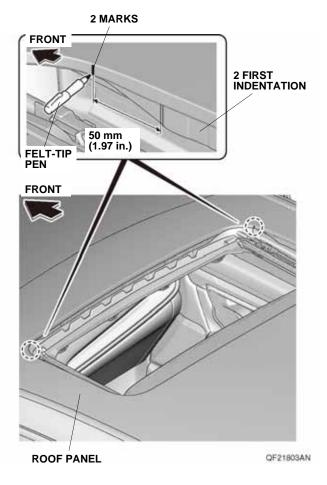
3. Using an alcohol swab, thoroughly clean the roof panel at each of the two marks you have made, but do not wipe off the marks.
