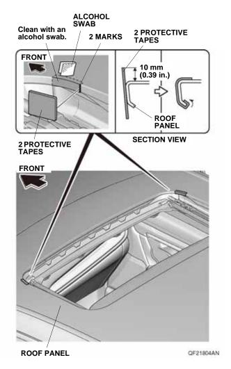
Remove the adhesive backing from the two protective tapes, and attach one to the roof panel at each of two marks you made. Wrap 10 mm (0.39 in.) of protective tape around the lip of the moonroof opening.  Locate the first indentations from the right front corner and left front corner of the moonroof opening. Using an alcohol swab, thoroughly clean the roof panel where the protective tapes will attach.
