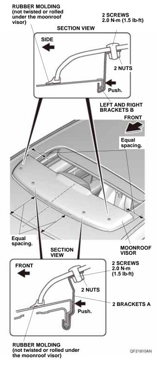
12. Tighten the two screws and two nuts on the front of the vehicle first, then tighten the two screws and two nuts on each side. Tighten while applying pressure so that there is no gap between the roof panel and brackets A and B. Torque the screws to 2.0 N·m (1.5 lb·ft).
