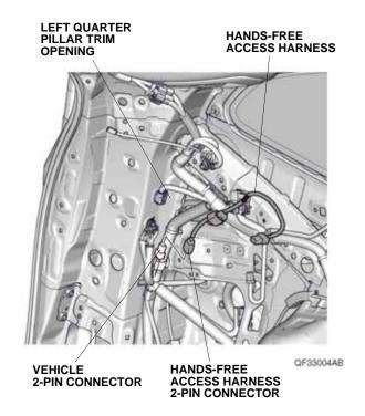
38. Line up the green tape on the hands-free access harness to the vehicle clip, and secure the hands-free access harness to the vehicle harness with one wire tie.
