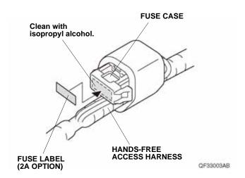
37. Plug the vehicle 2-pin connector into the hands-free access harness 2-pin connector.
