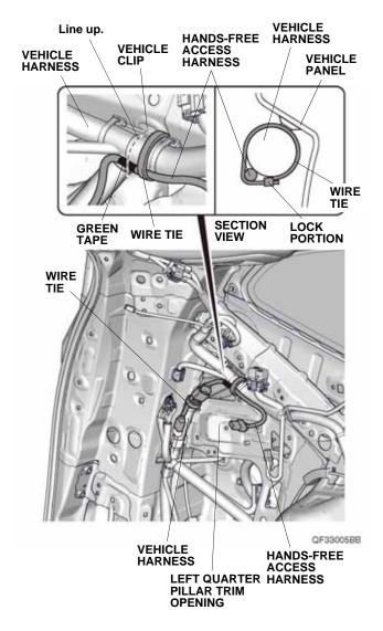
39. Secure the hands-free access harness to the vehicle harness with one wire tie.
