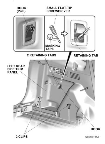
13. Apply masking tape to the left rear side trim panel as shown.
