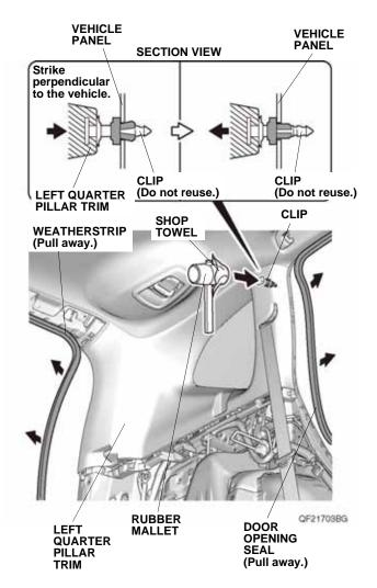
18. Using a rubber mallet wrapped with a shop towel, lightly tap the area marked **SIDE CURTAIN AIRBAG** on the left quarter pillar trim to push in the clip. Make sure to strike the area perpendicular to the vehicle.
