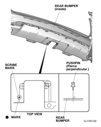
26. While wearing eye protection, drill the pierced mark on the rear bumper with a 3 mm drill bit. NOTE: Make sure to drill perpendicular to the rear bumper.
