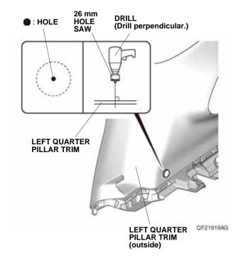
44. Install the switch into the 26 mm hole in the left guarter pillar trim.
