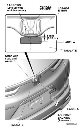
56. Remove the adhesive backing from the label A. Using the arrows on the label A, center it 5 mm (0.20 in.) below the tailgate trim and attach it to the tailgate.
