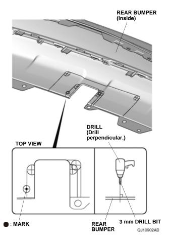
27. While wearing eye protection, enlarge the 3 mm hole to 14 mm using a 14 mm hole saw. Remove any burrs.
