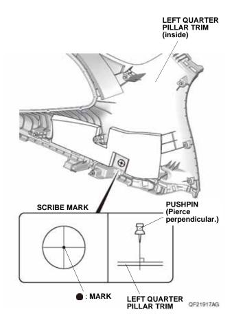
42. While wearing eye protection, drill the pierced mark on the left quarter pillar trim with a 3 mm drill bit. NOTE: Make sure to drill perpendicular to the left quarter pillar trim.
