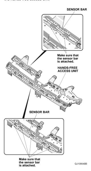
29. Install the hands-free access unit to the rear bumper with two self-tapping screws, three bumper clips A, one bumper clip B and one clip.
