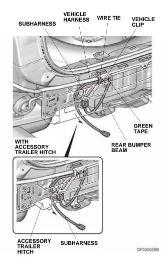
33. With the help of an assistant, bring the rear bumper close to the vehicle, and plug the subharness 3-pin connector into the hands-free access unit. Install the rear bumper.
