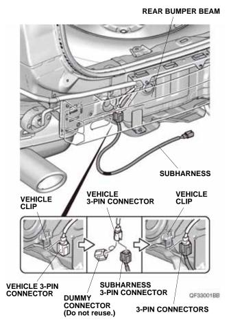
31. Plug the vehicle 3-pin connector into the subharness 3-pin connector, and secure the 3-pin connectors to the vehicle clip.
