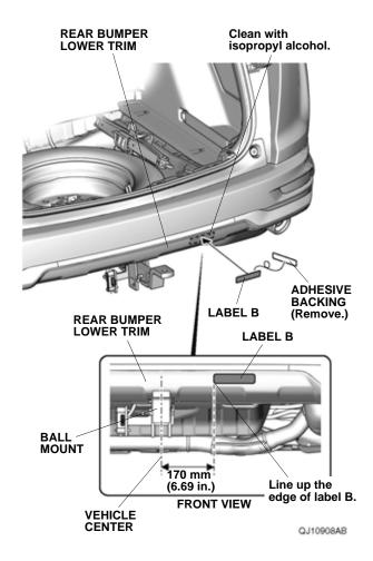
35. Remove the adhesive backing from the label B, and attach the label B to the rear bumper lower trim at the measurement shown.
