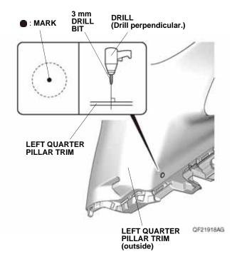
43. While wearing eye protection, enlarge the 3 mm hole to 26 mm using a 26 mm hole saw. Remove any burrs.
