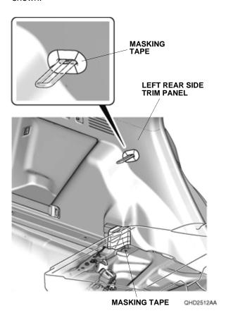
14. Pull away the door opening seal and weatherstrip from around the left rear side trim panel. Remove the left rear side trim panel, and unplug the vehicle connector.
