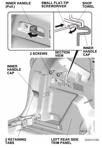
Remove the two screws from the left rear side trim panel. 12. Gently pull the hook on the left rear side trim panel, and use a small flat-tip screwdriver wrapped with masking tape to remove the hook as shown. Then, remove the two clips from the left rear side trim panel.
