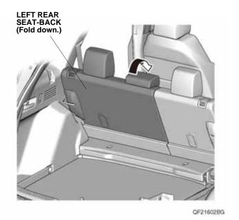
5. Remove the cargo floor board.
