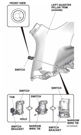
45. Line up the tab on the switch bracket with the hole on the switch, and secure the switch bracket to the switch with one narrow wire tie.
