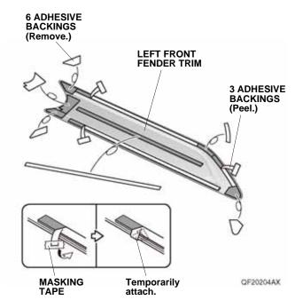
4. Line up the left front fender trim with the template, and attach it to the left front fender as shown.
