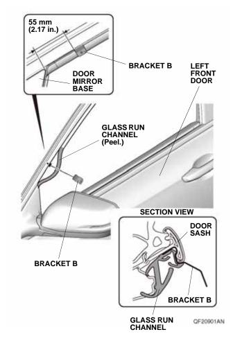
Install bracket B between the door sash and the glass run channel as shown. Seat the glass run channel properly around the bracket. NOTE: Confirm bracket B is installed on the door sash as shown. Check that the glass run channel is seated properly. 6. Use one alcohol swab to thoroughly clean the area where the left front door visor will attach.
