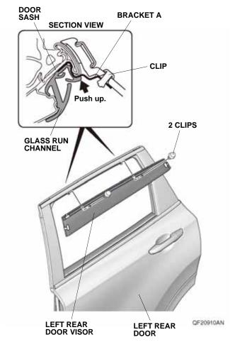
19. Using two clips secure the left rear door visor to the brackets as shown. Make sure to push up on the brackets while installing two clips.
