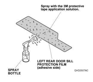
18. Line up the left rear door sill protection film with the curve end and masking tape as shown. Attach the left rear door sill protection film to the vehicle panel.
