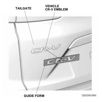
24. Attach the masking tape along the guide form as shown.
