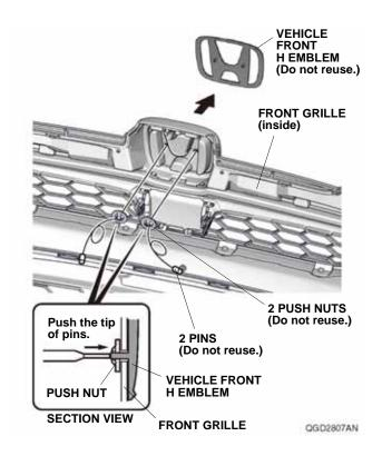
14. Using an alcohol wipe, thoroughly clean the front grille where the front H emblem will attach.
