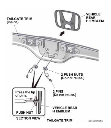
19. Using an alcohol wipe, thoroughly clean the tailgate trim where the rear H emblem will attach.
