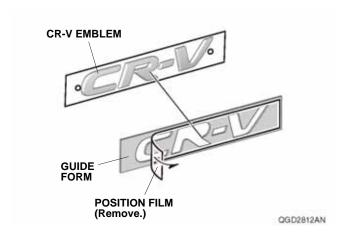
23. Install the guide form to the vehicle CR-V emblem on the tailgate.
