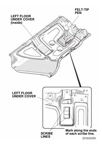
12. Using a utility knife, cut the left floor under cover as shown.
