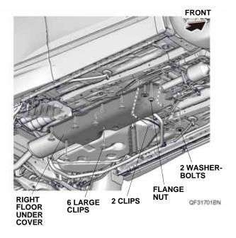
If the vehicle is equipped with the insulator on the floor under covers, continue with step 8; otherwise, go to step 10.
