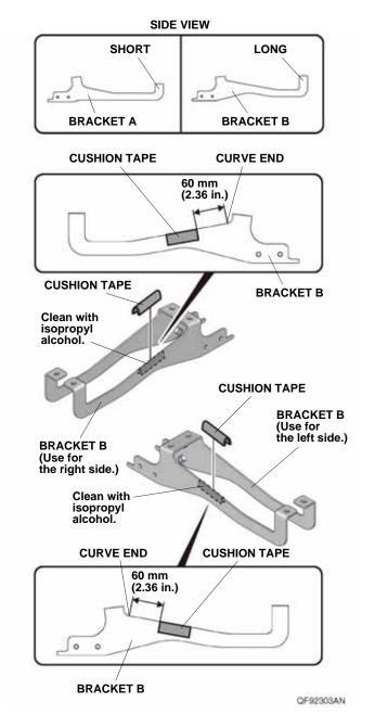
17. Attach one cushion tape to each bracket B as shown. Make sure to attach the cushion tapes in the correct position and orientation.
