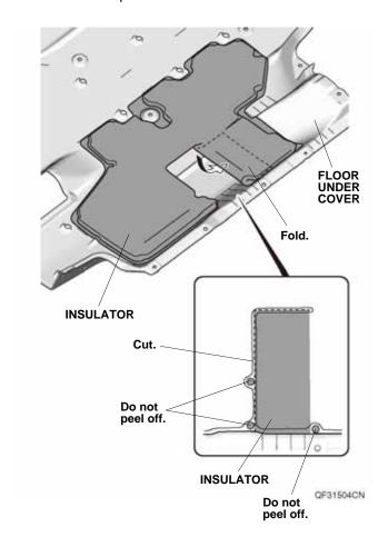
4. Using a utility knife, cut off the floor under cover as shown.
