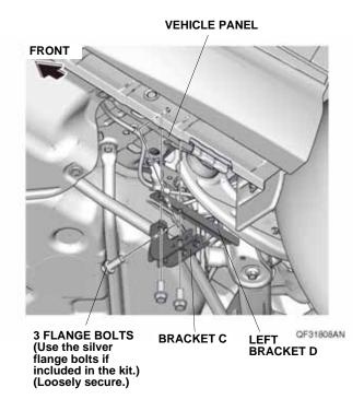
26. With the help of an assistant, loosely secure the left running board to bracket A, bracket B, bracket C, and left bracket D with 13 flange bolts.
