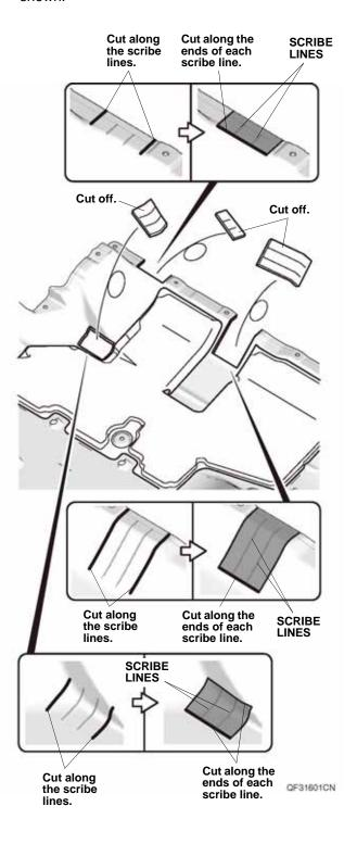
5. Using a utility knife, cut off the floor under cover as shown. Go to step 16.
