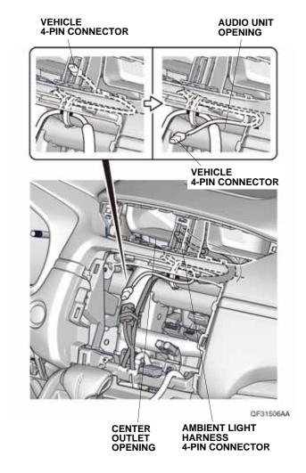
15. Plug the vehicle 4-pin connector into the ambient light harness 4-pin connector.
