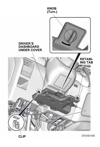
7. Remove the driver's dashboard lower cover and unplug the vehicle connectors.
