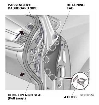
3. Remove the passenger's dashboard under cover.
