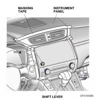
Remove the center outlet and unplug the vehicle connector.
