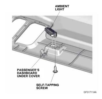
33. Install the glove box. Plug the ambient light harness 4-pin connector into the ambient light, then install the passenger's dashboard under cover.
