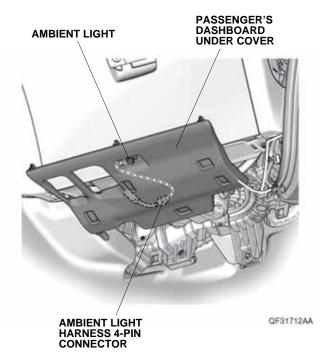
34. Install the audio unit and climate control unit. Plug the ambient light harness 4-pin connector into the center outlet, then install the center outlet.
