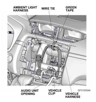
14. Route the vehicle 4-pin connector and ambient light harness 4-pin connector as shown.
