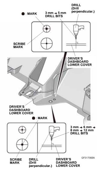
27. While wearing eye protection, drill the pierced mark on the driver's dashboard lower cover to 12 mm. First drill with a 3 mm drill bit, next drill with a 6 mm drill bit and an 8 mm drill bit, and finish with a 12 mm drill bit. Remove any burrs.
