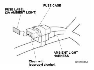
13. Line up the edge of green tape on the ambient light harness with the clip on the vehicle harness and secure the ambient light harness to the vehicle harness with one wire tie as shown.
