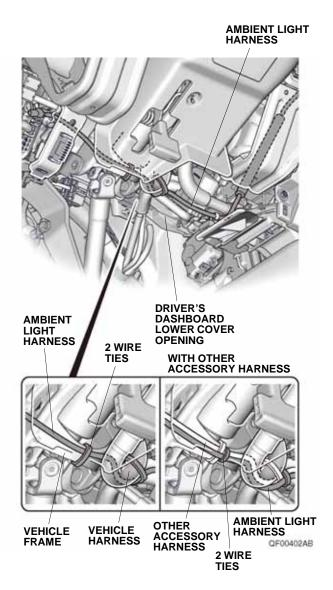
21. Secure the ambient light harness to the vehicle harness with one wire tie. Move the steering wheel up and down through its full adjustment range and make sure the ambient light harness is not being pinched or stretched.
