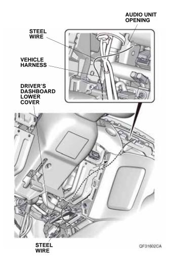
18. Attach the steel wire to the ambient light harness with tape and route the harness as shown.
