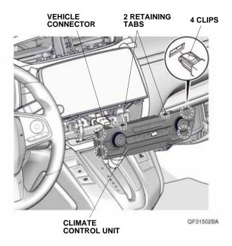
Remove the audio unit and unplug the vehicle connectors.
