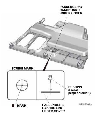
31. While wearing eye protection, drill the pierced mark on the passenger's dashboard under cover to 5 mm. First drill with a 3 mm drill bit and finish with a 5 mm drill bit. Remove any burrs.
