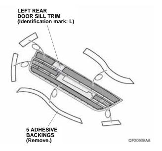
26. Line up the left rear door sill trim with the masking tape attached in step 13, and install the left rear door sill trim to the vehicle panel.
