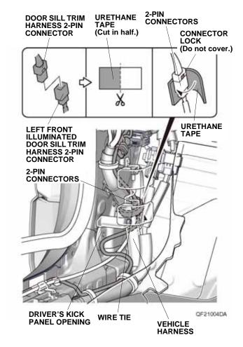
37. Using scissors, cut one urethane tape in half, and attach one half of urethane tape around the 2-pin connectors.
