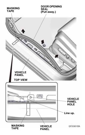
Using an alcohol swab, thoroughly clean the vehicle panel where the left front illuminated door sill trim will attach.
