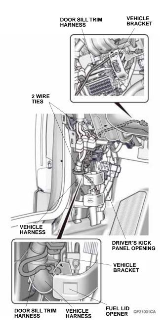
32. Peel back the floor carpet, and route the left front illuminated door sill trim harness as shown.
