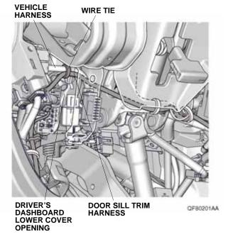
43. Route the door sill trim harness as shown, and secure it to the vehicle panel with one clip on the door sill trim harness.
