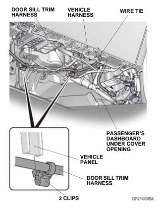
46. Secure the door sill trim harness to the vehicle harness with one wire tie.
