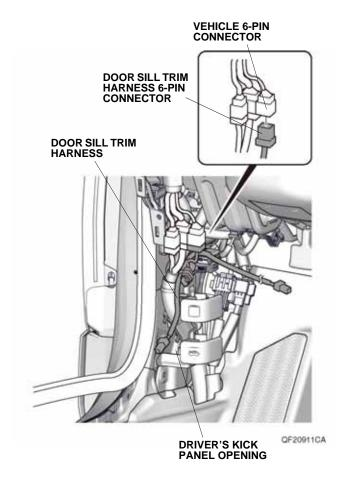
31. Route the door sill trim harness as shown, and secure the door sill trim harness to the vehicle harness with two wire ties.
