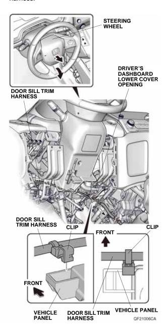
41. Secure the door sill trim harness to the vehicle frame and vehicle harness with two wire ties. If the vehicle is already equipped with the other accessory harness, secure the door sill trim harness to the other accessory harness with two wire ties as shown.
