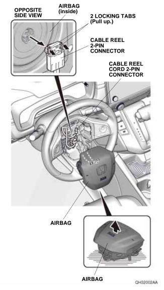
Remove the airbag. Do not drop the removed airbag or hit it on an object. Place the removed airbag in a safe place with the padded surface (top) facing up. 11. With the front wheels line up in the straight-ahead position, unplug the vehicle connector from the cable reel, and loosen the steering wheel bolt.
