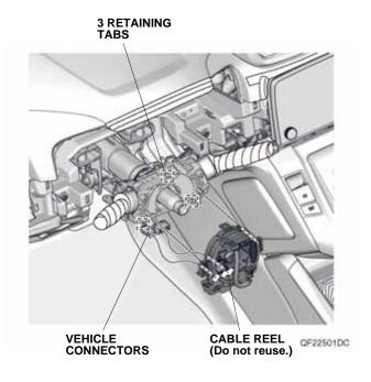
28. Install the new cable reel with three retaining tabs, and plug the vehicle connectors into the new cable reel.
