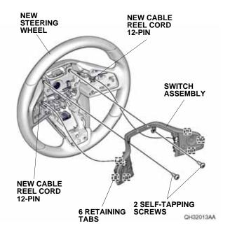
51. Install the control unit on the steering wheel trim with two self-tapping screws.
