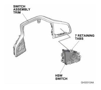
50. Plug the two new cable reel cord 12-pin connectors into the switch assembly, and install the switch assembly on the new steering wheel with six retaining tabs and two self-tapping screws removed in step 42.
