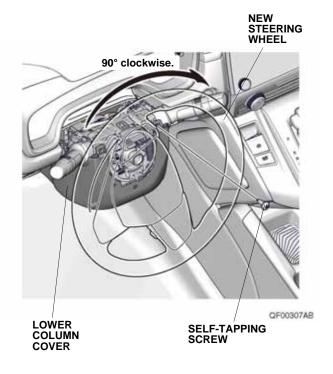
63. Turn the new steering wheel 180° counterclockwise. Secure the lower column cover.
