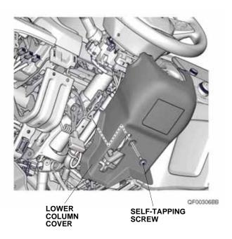
62. Connect the negative cable to the battery, then turn the engine switch to ON. Turn the new steering wheel 90° clockwise. Secure the lower column cover.
