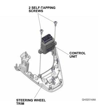
52. Plug the new cable reel cord 14-pin connector into the control unit, and install the steering wheel trim on the new steering wheel with two retaining tabs and two self-tapping screws removed in step 42.
