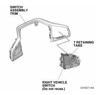
49. Install the HSW switch on the switch assembly trim with seven retaining tabs.
