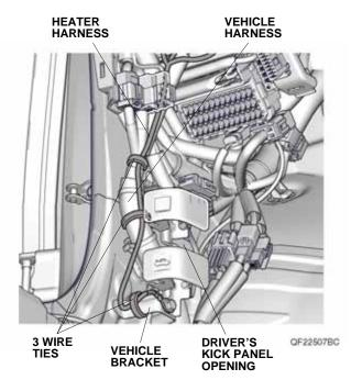
34. Route the heater harness along the vehicle harness, and secure it to the vehicle harness with two wire ties.
