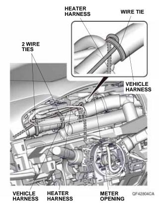
40. Secure the heater harness to the vehicle harnesses with two wire ties.
