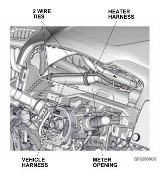
36. Route the heater harness along the driver's dashboard lower cover opening as shown.
