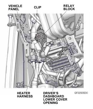
31. Plug the heater harness 4-pin connector into the fuse box.
