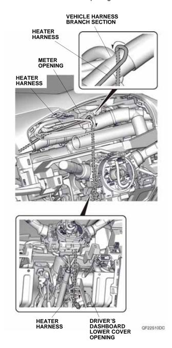
37. Route the heater harness along the vehicle harness, and secure it to the vehicle harness with two wire ties at the green tapes on the heater harness.
