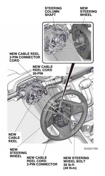
56. Install the new steering wheel bolt. Torque the new steering wheel bolt to 36 lb-ft (49 N·m). Tighten to the specified torque within 5 minutes.
