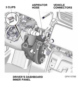
25. Remove the meter, and unplug the vehicle connectors.
