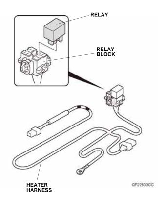
30. Install the relay block on the heater harness to the vehicle panel with clip on the relay block.
