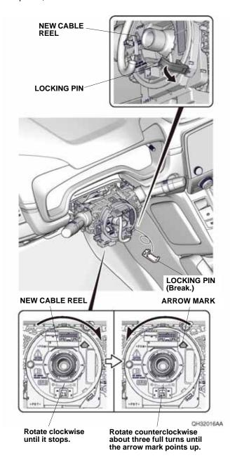
54. Break the locking pin as direction shown. Before installing the new steering wheel, make sure the front wheels are still pointing straight-ahead. To confirm the cable reel is line up properly, rotate the cable reel clockwise until it stops, then rotate it counterclockwise about three full turns. The arrow mark on the new cable reel label must point straight up.
