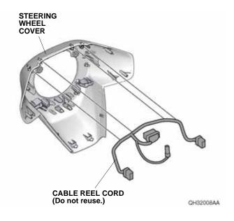
Install the new cable reel cord on the steering wheel cover.
