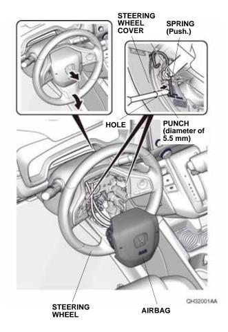
8. Insert a punch (diameter of 5.5 mm) through the left hole of the steering wheel cover, and push the spring to release the airbag. Repeat for the other side.
