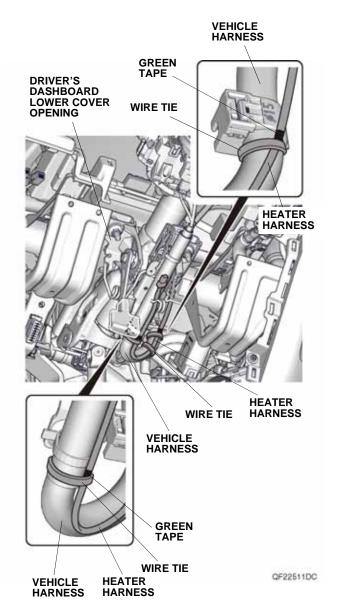
38. Secure the heater harness to the vehicle harness with one wire tie.
