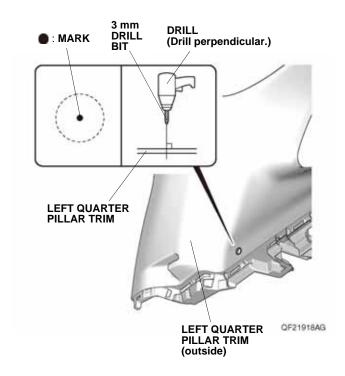
60. While wearing eye protection, enlarge the 3 mm hole to 26 mm using a 26 mm hole saw. Remove any burrs
