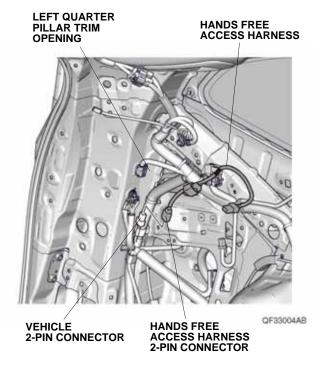
42. Line up the green tape on the hands free access harness to the vehicle clip, and secure the hands free access harness to the vehicle harness with one wire tie.
