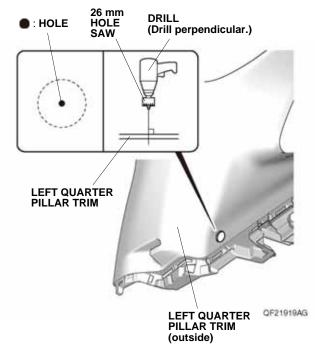
61. Install the switch into the 26 mm hole in the left guarter pillar trim.
