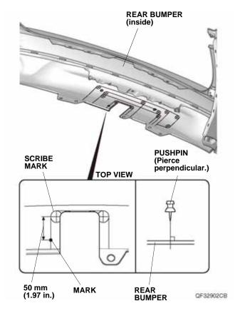
24. While wearing eye protection, drill the pierced mark on the rear bumper with a 3 mm drill bit. NOTE: Make sure to drill perpendicular to the rear bumper.
