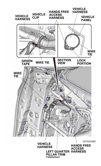
43. Secure the hands free access harness to the vehicle harness with one wire tie.
