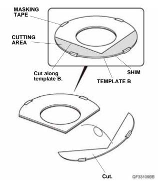
54. Using scissors, cut the shim along template B as shown. Remove the template B.
