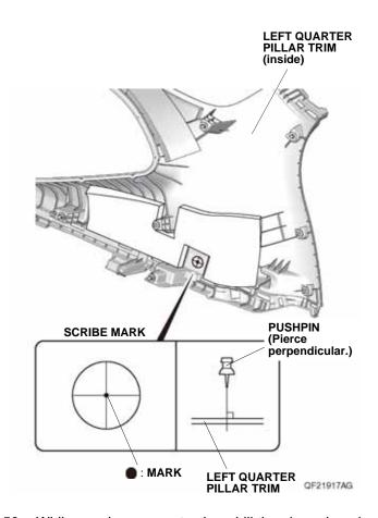
59. While wearing eye protection, drill the pierced mark on the left quarter pillar trim with a 3 mm drill bit. NOTE: Make sure to drill perpendicular to the left quarter pillar trim.
