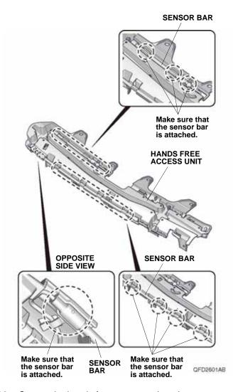
32. Secure the hands free access unit to the accessory rear aero bumper with two self-tapping screws, one bumper clip A, and four bumper clips B. Go to step 34.
