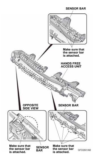
27. Secure the hands free access unit to the rear bumper with two self-tapping screws, one bumper clip A, and four bumper clips B. Go to step 34.
