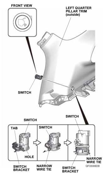
62. Line up the tab on the switch bracket with the hole on the switch, and secure the switch bracket to the switch with one narrow wire tie.
