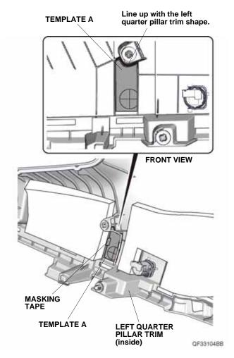
49. Using a pushpin, pierce the mark in template A. Remove the template.
