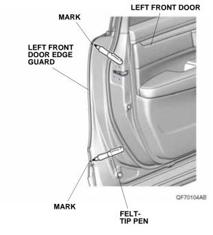
3. Remove the left front door edge guard. 4. Position the cutting edge of the seam sealant cutting tool against the door edge, and carefully trim the seam sealant from mark to mark. NOTE: The cutting tool cuts in only one direction.
