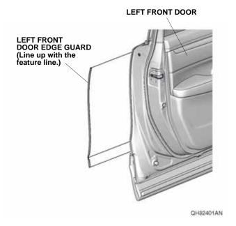
2. Mark the sealant at the top and bottom edges of the left front door edge guard.
