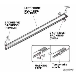
7. Line up the left front body side molding with the front template, and attach it to the left front door as shown.
