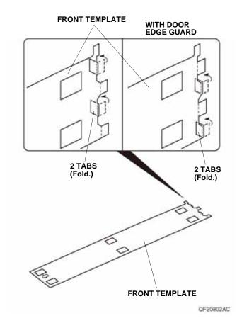
2. Insert the folded tabs on the front template between the left front door and left rear door. Line up the front template with the left front door lower trim, and attach it to the left front door with masking tape.
