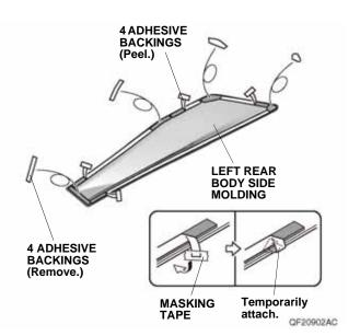
12. Line up the left rear body side molding with the rear template, and attach it to the left rear door as shown.
