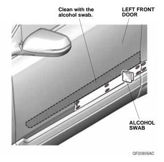
5. Using one alcohol swab, thoroughly clean the left rear door where the left rear body side molding will attach.
