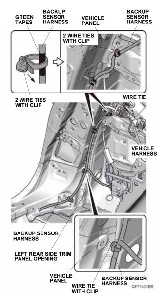
48. Secure the backup sensor harness to the vehicle harness and vehicle panel with one wire tie and one wire tie with clip.
