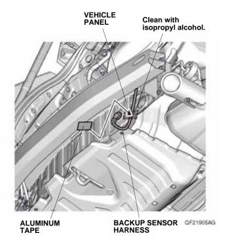
60. Secure the backup sensor harness to the vehicle panel with one aluminum tape as shown.
