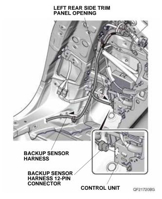
If the other harness is installed in the area shown, continue with step 44; otherwise, go to step 47.
