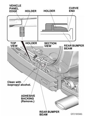
57. Remove the adhesive backing from the holder, and attach the holder as shown.
