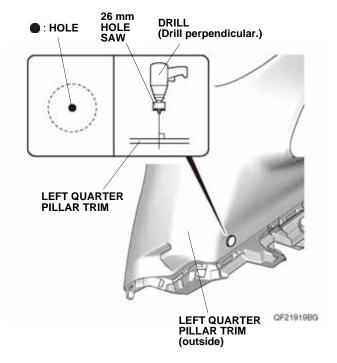
82. Install the switch into the 26 mm hole in the left guarter pillar trim.
