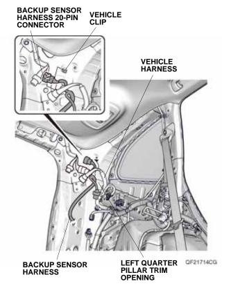
32. Plug the vehicle 20-pin connector into the backup sensor harness 20-pin connector. Plug the remaining backup sensor harness 20-pin connector into the vehicle 20-pin connector.
