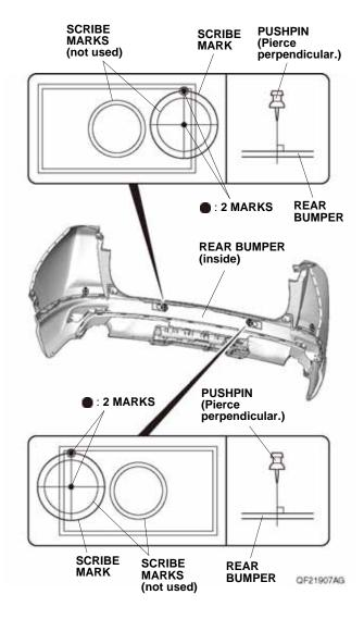
63. While wearing eye protection, drill the eight pierced marks with a 3 mm drill bit from the painted side of the rear bumper.
