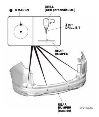
64. While wearing eye protection and drilling from the painted side of the rear bumper, enlarge the two lower 3 mm outer holes to 24 mm using a 24 mm hole saw.
