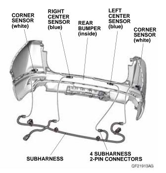
74. Secure the clips on the subharness to the right center sensor clip (green), left center sensor clip (white), and ribs on the rear bumper.
