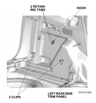
13. Pull away the door opening seal and weatherstrip from around the left rear side trim panel. Remove the left rear side trim panel, and unplug the vehicle connector.
