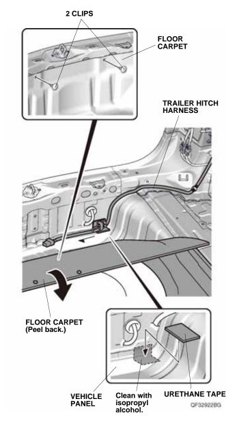
84. Using isopropyl alcohol on a shop towel, thoroughly clean the vehicle panel where the urethane tape will attach. Attach the urethane tape to the vehicle panel as shown.
