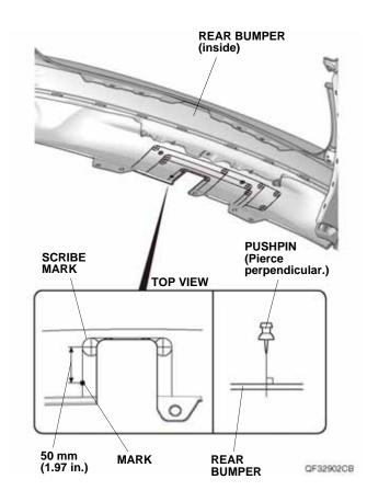
While wearing eye protection, drill the pierced mark on the rear bumper with a 3 mm drill bit.
