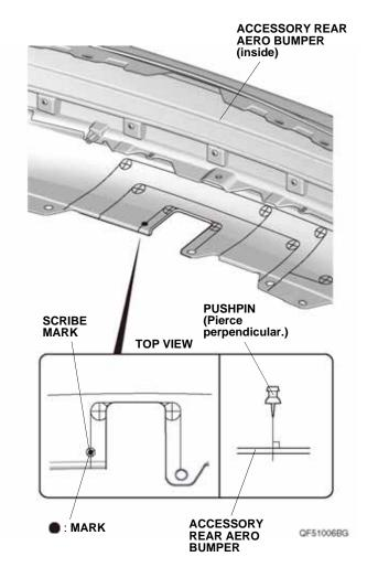
48. While wearing eye protection, drill the pierced mark on the accessory rear aero bumper with a 3 mm drill bit
