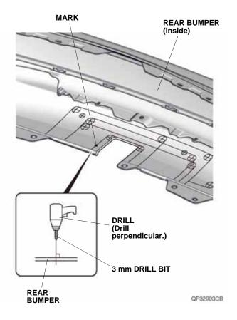
40. While wearing eye protection, enlarge the 3 mm hole to 14 mm using a 14 mm hole saw. Remove any burrs.
