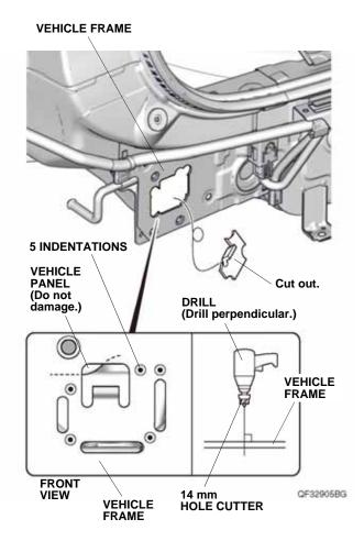
52. Using a file, file the vehicle frame as shown.
