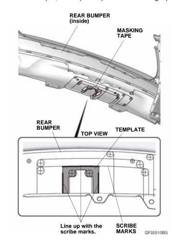
32. Using a felt-tip pen, mark the rear bumper along the template.
