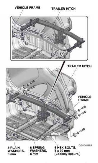
58. Loosely secure the trailer hitch to the vehicle frame with six 8 mm plain washers, six 8 mm spring washers, and six 8 x 30 mm hex bolts.
