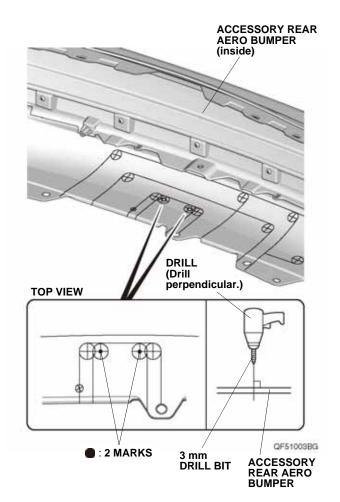
45. While wearing eye protection, enlarge the 3 mm holes to 20 mm using a 20 mm hole saw. Remove any burrs.
