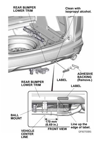
93. Remove the adhesive backing from the label, and attach the label to the rear bumper lower trim as shown.
