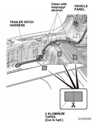
86. Using scissors, cut two aluminum tapes in half, and secure the trailer hitch harness to the vehicle panel with three halves of aluminum tape as shown.
