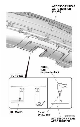
49. While wearing eye protection, enlarge the 3 mm hole to 14 mm using a 14 mm hole saw. Remove any burrs
