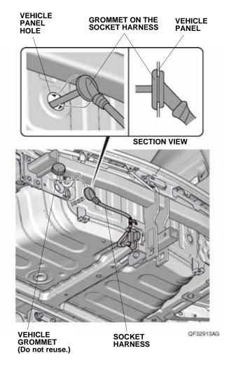
67. Install the grommet on the socket harness into the vehicle panel hole.
