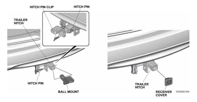
After the first 600 miles (1,000 km) of towing, have your Honda dealer check the tightness of the trailer hitch bolts.
