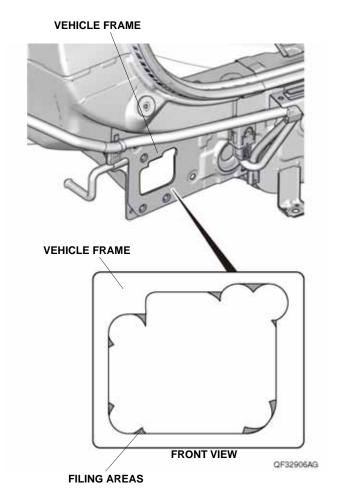
53. Apply touch-up paint to the edges of the holes. Allow the touch-up paint to dry thoroughly.
