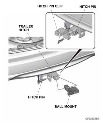
91. Secure the ball mount to the trailer hitch with the hitch pin and hitch pin clip.
