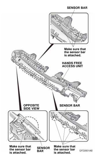
42. Install the hands free access unit to the rear bumper with two self-tapping screws, four clips, and one bumper clip. Go to step 51.
