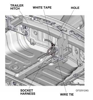
66. Remove the vehicle grommet. Route the socket harness through the vehicle panel hole.
