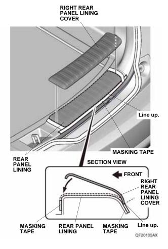
Using a rubber roller, apply firm pressure against the right rear panel lining cover, and roll from one end to the other. Apply firm pressure, especially at the ends.
