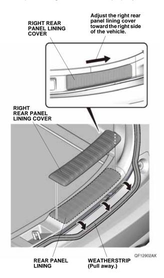
2. Attach masking tape along the right rear panel lining cover first, then remove the right rear panel lining cover from the rear panel lining.
