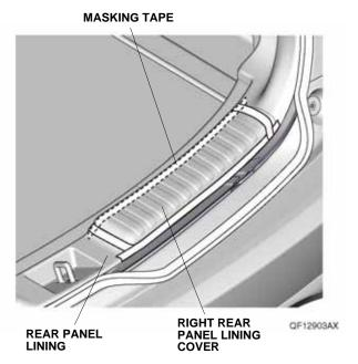
3. Using the alcohol swab, thoroughly clean the rear panel lining where the right rear panel lining cover will attach.
