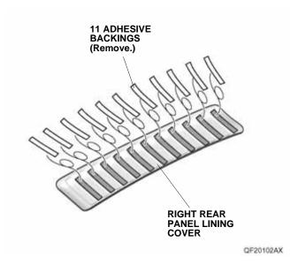
5. Line up the right rear panel lining cover with masking tape. Carefully attach the right rear panel lining cover from the rear toward the front of the vehicle as shown.
