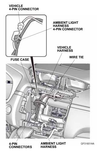
16. Secure the 4-pin connectors, fuse case, and ambient light harness to the vehicle harness with one wire tie as shown.
