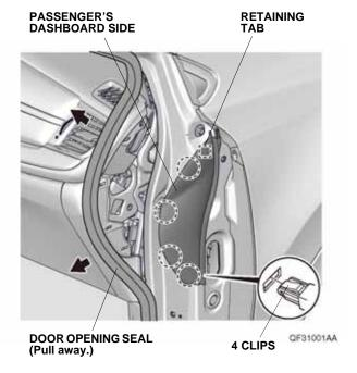
3. Remove the passenger's dashboard under cover.
