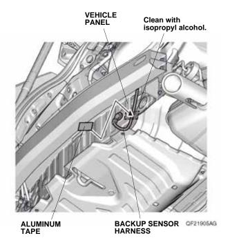
60. Secure the backup sensor harness to the vehicle panel with one aluminum tape as shown.
