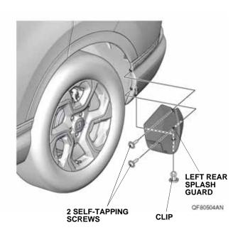
21. Remove the self-tapping screw from the left rear wheel arch protector.
