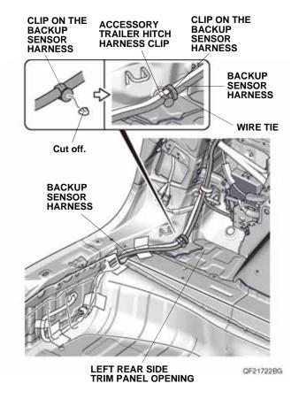
50. Secure the backup sensor harness to the accessory trailer hitch harness with one wire tie. Go to step 52.
