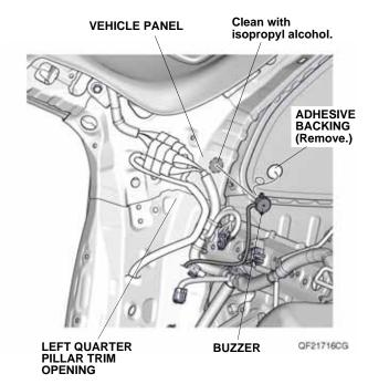
36. Remove the adhesive backing from the buzzer, and attach the buzzer to the vehicle panel as shown.
