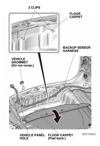
53. Secure the grommet on the backup sensor harness into the vehicle panel hole.
