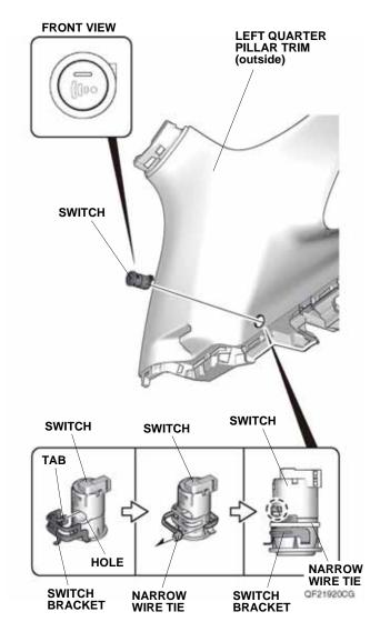
83. Line up the tab on the switch bracket with the hole on the switch, and secure the switch bracket to the switch with one narrow wire tie.
