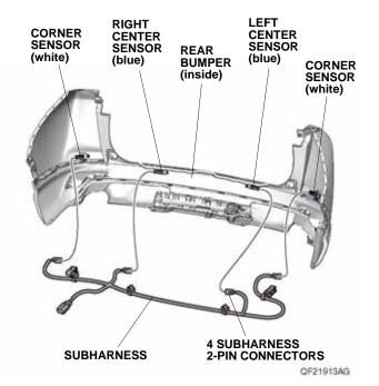
74. Secure the clips on the subharness to the right center sensor clip (green), left center sensor clip (white), and ribs on the rear bumper.
