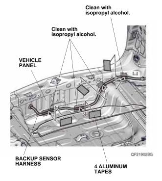
55. Secure the backup sensor harness to the vehicle panel with four aluminum tapes as shown.
