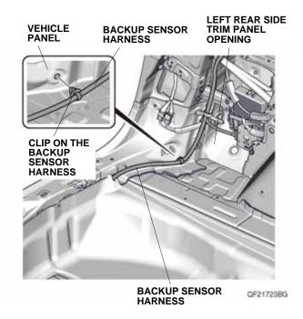
52. Peel back the floor carpet, then remove the vehicle grommet. Route the backup sensor harness through the vehicle panel hole.
