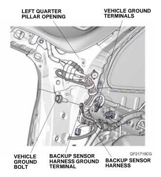
42. Secure the backup sensor harness ground terminal to the vehicle ground terminals with the vehicle ground bolt just removed. Do not put the ground terminal calkings on top of one another.
