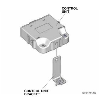
Secure the control unit bracket to the vehicle panel with one flange bolt.
