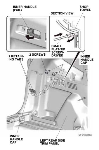
11. Remove the two screws from the left rear side trim panel.
