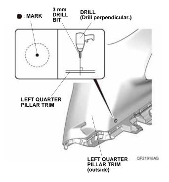
81. While wearing eye protection, enlarge the 3 mm hole to 26 mm using a 26 mm hole saw.
