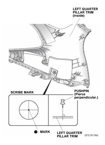
80. While wearing eye protection, drill the pierced mark on the left quarter pillar trim with a 3 mm drill bit. NOTE: Make sure to drill perpendicular to the left quarter pillar trim.
