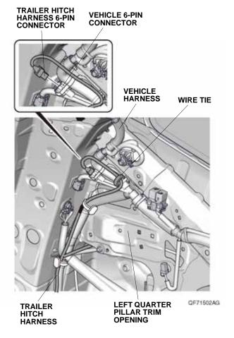
79. Secure the trailer hitch harness to the vehicle harness with one wire tie.
