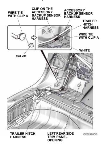
81. Line up the white tape on the trailer hitch harness to the clip on the accessory backup sensor harness, and secure the trailer hitch harness to the accessory backup sensor harness with one wire tie with clip A. Go to step 83.
