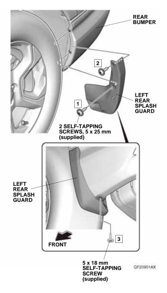
11. While holding the left rear splash guard against the rear bumper, tighten the two 5 x 25 mm self-tapping screws and one 5 x 18 mm self-tapping screw in the order shown.
