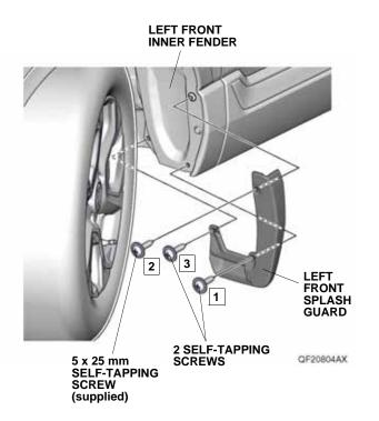
5. While holding the left front splash guard against the left front inner fender, tighten one 5 x 25 mm self-tapping screw and two self-tapping screws in the order shown.
