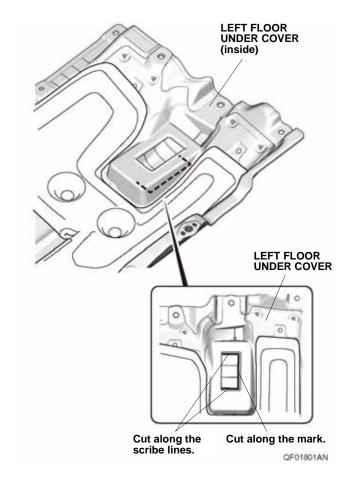
13. Using a felt-tip pen, mark the left floor under cover as shown.
