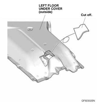
15. Using a utility knife, cut off the left floor under cover as shown.
