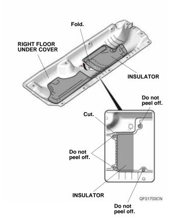
Using a utility knife, cut off the right floor under cover as shown.
