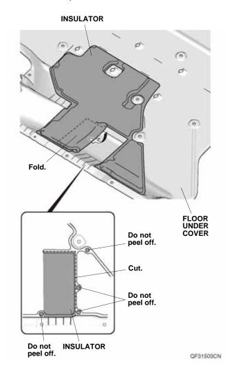
3. Using a utility knife, cut the insulator on the floor under cover and fold it into the inside of the insulator as shown
