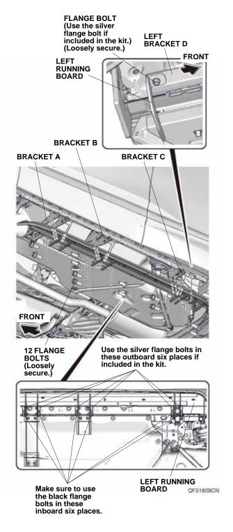
27. Secure bracket A, bracket B, and bracket C to the vehicle panel with nine flange bolts. Torque the flange bolts to 22 N·m (16 lb·ft).
