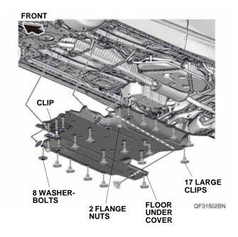
If the vehicle is equipped with the insulator on the floor under cover, continue with step 2; otherwise, go to step 4.
