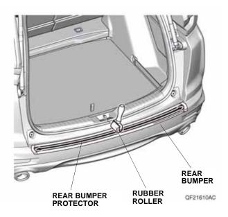
11. Remove the masking tape from the rear bumper and the sticker on the rear bumper protector.
