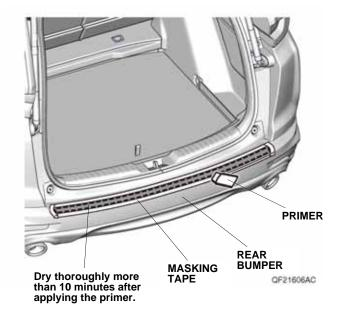
Peel back the adhesive backings, and tape them to the surface of the rear bumper protector with strips of masking tape. Remove the remaining adhesive backings.
