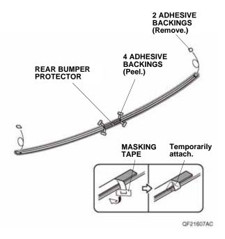
8. Align with masking tape, and attach the rear bumper protector as shown.
