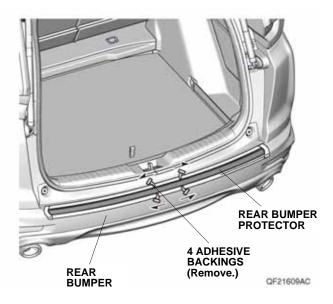
Using a rubber roller, apply firm pressure against the rear bumper protector and roll from one end to the other. Apply firm pressure, especially at the ends.
