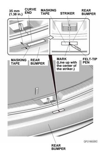
Line up the sticker on the rear bumper protector with the mark on masking tape as shown. Position the rear bumper protector on the rear bumper. Make sure that the rear end of the rear bumper protector is within the curve end of the rear bumper.
