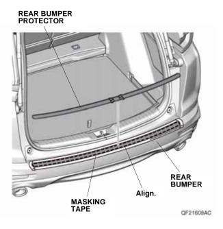
While applying light pressure against the rear bumper protector, carefully remove the taped adhesive backings.
