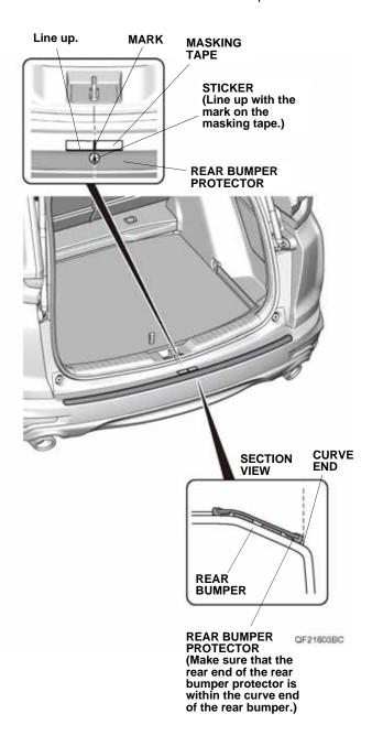
Attach masking tape along the rear bumper protector as shown.
