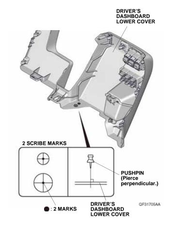
26. While wearing eye protection, drill the pierced mark on the driver's dashboard lower cover to 5 mm. First drill with a 3 mm drill bit and finish with a 5 mm drill bit. Remove any burrs.
