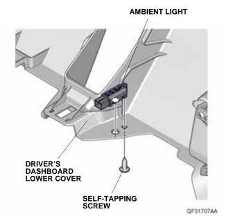
29. Plug the ambient light harness 4-pin connector into the ambient light, then install the driver's dashboard lower cover.
