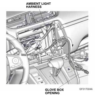
23. Line up the green tape on the ambient light harness with the edge of the vehicle frame as shown. Secure the ambient light harness to the vehicle frame with two wire ties.
