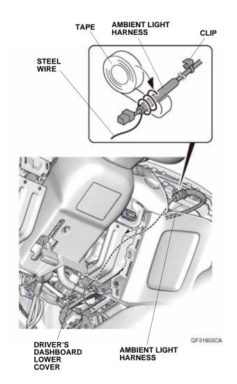
19. Lower and pull out the steering wheel. Route the ambient light harness as shown. Remove the tape and steel wire. Secure the ambient light harness to the vehicle panel with one clip on the ambient light harness.
