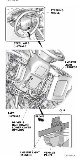
20. Secure the ambient light harness to the vehicle frame and vehicle harness with two wire ties. If the vehicle is already equipped with the other accessory harness, secure the ambient light harness to the other accessory harness with two wire ties as shown.
