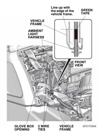
24. Secure the ambient light harness to the vehicle harness and vehicle frame with two wire ties.
