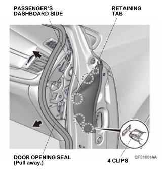
3. Remove the passenger's dashboard under cover.
