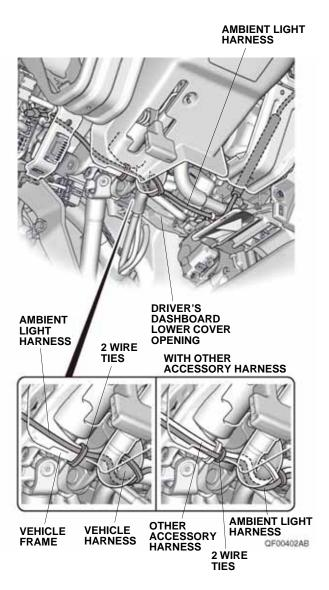
21. Secure the ambient light harness to the vehicle harness with one wire tie. Move the steering wheel up and down through its full adjustment range and make sure the ambient light harness is not being pinched or stretched.
