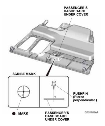
31. While wearing eye protection, drill the pierced mark on the passenger's dashboard under cover to 5 mm. First drill with a 3 mm drill bit and finish with a 5 mm drill bit. Remove any burrs.
