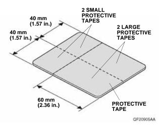
21. Using isopropyl alcohol on a shop towel, thoroughly clean the vehicle panel where the small protective tape will attach. Attach one piece of small protective tape to the vehicle panel as shown.
