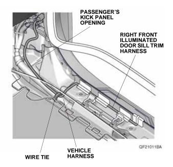
51. Plug the door sill trim harness 2-pin connector into the right front illuminated door sill trim harness 2-pin connector.
