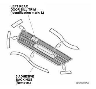
26. Line up the left rear door sill trim with the masking tape attached in step 13, and install the left rear door sill trim to the vehicle panel.
