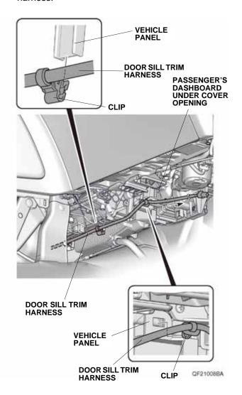
45. Route the door sill trim harness, and secure it to the vehicle panel with two clips on the door sill trim harness.
