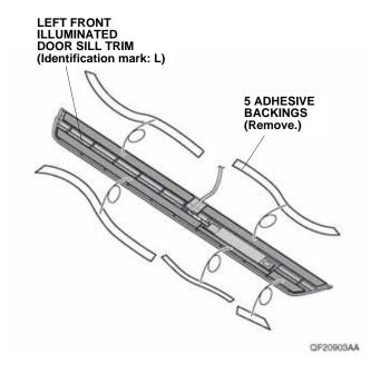
18. Line up the left front illuminated door sill trim with the masking tape attached in step 15, and install the left front illuminated door sill trim to the vehicle panel.
