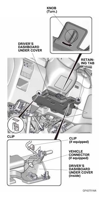
9. Remove the driver's dashboard lower cover and unplug the vehicle connectors.
