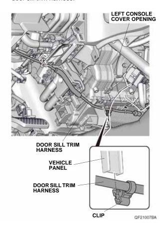
44. Route the door sill trim harness, and secure it to the vehicle panel with two clips on the door sill trim harness.
