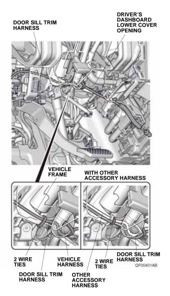
42. Secure the door sill trim harness to the vehicle harness with one wire tie. Move the steering wheel up and down through its full adjustment range and make sure the door sill trim harness is not being pinched or stretched.
