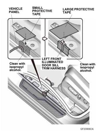
22. Using isopropyl alcohol on a shop towel, thoroughly clean the small protective tape where the large protective tape will attach. Secure the left front illuminated door sill trim harness to the vehicle panel with the large protective tape as shown.
