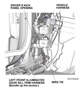
40. Lower and pull out the steering wheel. Route the door sill trim harness as shown, and secure it to the vehicle panel with one clip on the door sill trim harness.
