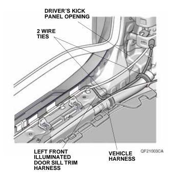
36. Plug the door sill trim harness 2-pin connector into the left front illuminated door sill trim harness 2-pin connector.
