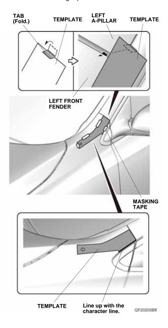
Peel back the adhesive backings, and tape them to the front surface of the left front fender trim with masking tape. Remove the remaining adhesive backings.
