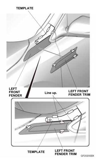
5. While applying light pressure against the left front fender trim, carefully remove the taped adhesive backings.
