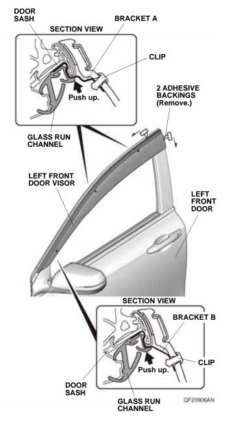
12. Using a soft towel; press and hold the left front door visor against the door sash for 30 seconds.
