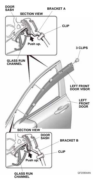
Using three clips secure the left front door visor to the brackets as shown. Make sure to push up on the brackets while installing three clips.
