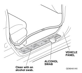
26. Align the right front illuminated door sill trim with the masking tapes and install the right front illuminated door sill trim to the vehicle panel.
