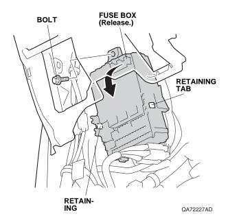
39. Using isopropyl alcohol on a shop towel, thoroughly clean the fuse case where the fuse label will attach. Attach the fuse label (2A STEP ILLUMI) to the fuse case on the door sill trim harness.
