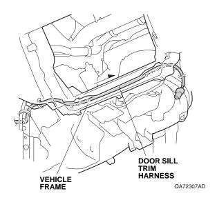
56. Using isopropyl alcohol on a shop towel, thoroughly clean the vehicle panel where the aluminum tapes will attach.
