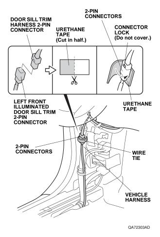
50. Using scissors, cut one urethane tape in half, and attach one piece of urethane tape around the 2-pin connectors.
