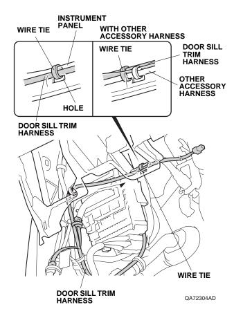
Route the door sill trim harness, and secure it to the vehicle frame with one wire tie.
