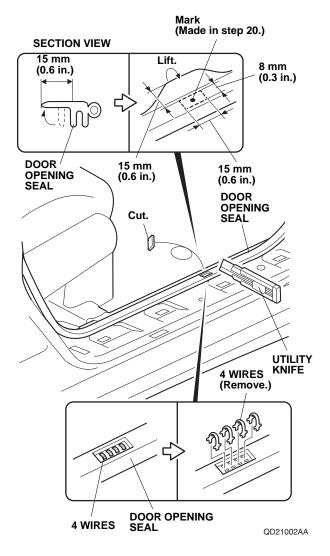
23. Remove the four wires from the part of the door opening seal.
