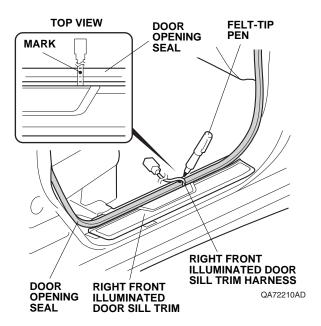
21. Pull away the door opening seal, and remove the right front illuminated door sill trim.
