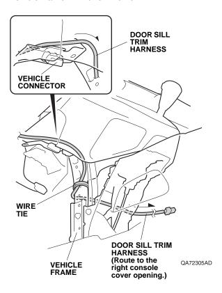
54. Route the door sill trim harness, and secure it to the vehicle frame with two wire ties.
