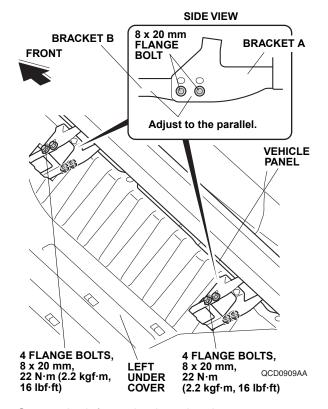
49. Secure the left running board to the two brackets A. Torque the flange bolts: 22 N·m (2.2 kgf·m, 16 lbf·ft).
