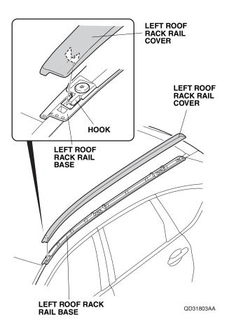
16. Secure the left roof rack rail cover to the left roof rack base with eight clips.
