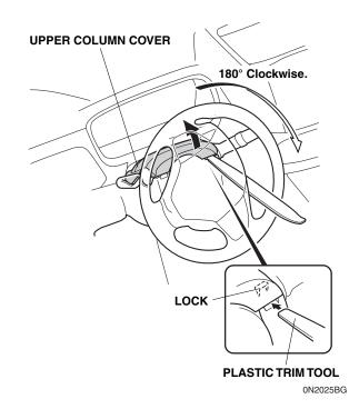
8. Secure the upper column cover to the meter panel with the tape.
