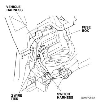
52. Unplug the vehicle connector from the light switch.
