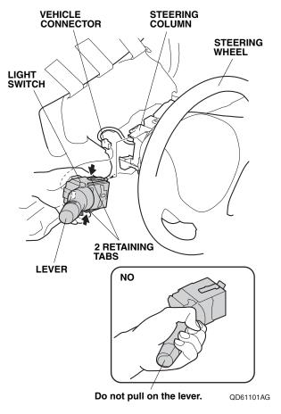
53. Push in on the two retaining tabs, slide the light switch out, and remove it from the steering column. Do not pull on the lever.
