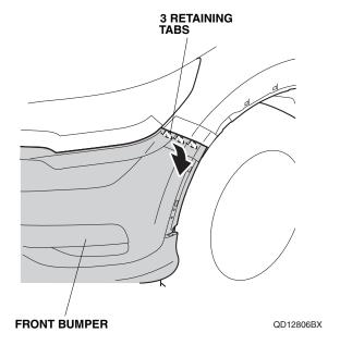
On each side, release the four retaining tabs.
