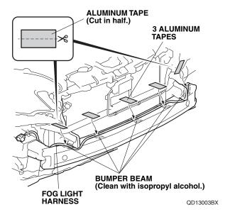
34. Using scissors, cut one aluminum tape in half.
