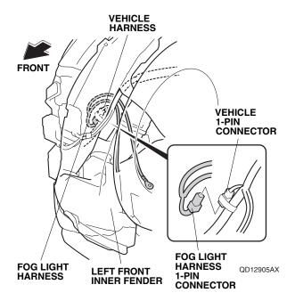
27. Secure the fog light harness to the vehicle harness with two wire ties.
