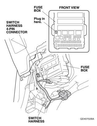
45. Plug the switch harness 4-pin connector to the fuse box. Go to step 48.
