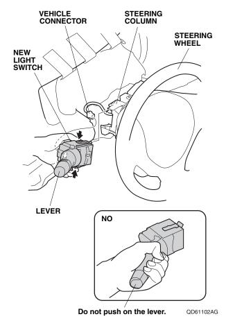
55. Plug the vehicle connector to the new light switch. Make sure the vehicle harness is not being stretched.
