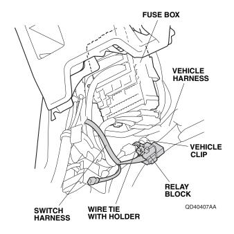
43. Plug the switch harness 1-pin connector to the vehicle 1-pin connector.
