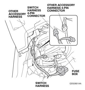
47. Plug the switch harness 4-pin connector to the other accessory harness 4-pin connector.
