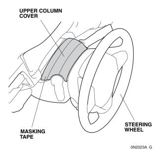
Lower the tilt lever, and turn the steering wheel 90° counterclockwise.
