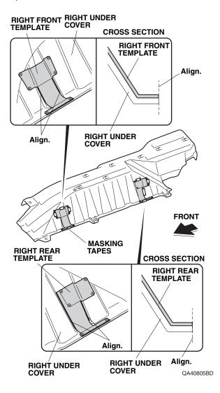
24. Using a pushpin, pierce six marks on the each templates.
