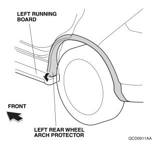
51. Secure the left running board to the left rear wheel arch protector with two self-tapping screw removed in step 4.
