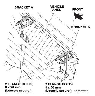
45. With help from an assistant, loosely secure the left running board to the two brackets A using four 8 x 20 mm flange bolts.
