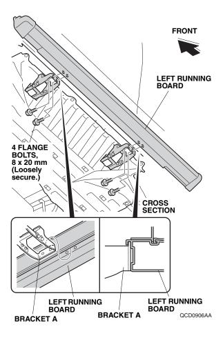
46. Secure the two brackets B to the vehicle panel. Torque the flange bolts: 22 N·m (2.2 kgf·m, 16 lbf·ft).
