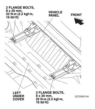
47. Secure the two brackets A to the vehicle panel. Torque the flange bolts: 22 N·m (2.2 kgf·m, 16 lbf·ft).
