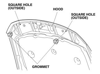
4. Using an alcohol swab, thoroughly clean the hood where the protective tapes will attach.
