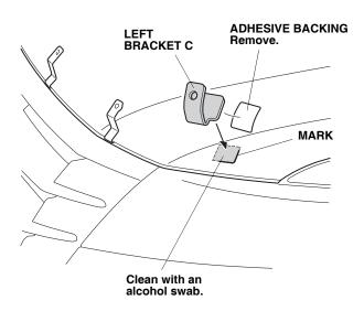
10. Turn the template over and repeat steps 7 thru 9 to install the right bracket C on the right side of the vehicle.
